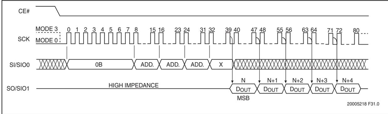
In SQI protocol, the host drives CE# low then send the Read command cycle command, 0BH, followed by three address cycles, a Set Mode Configuration cycle, and two dummy cycles. Each cycle is two nibbles (clocks) long, most significant nibble first.
