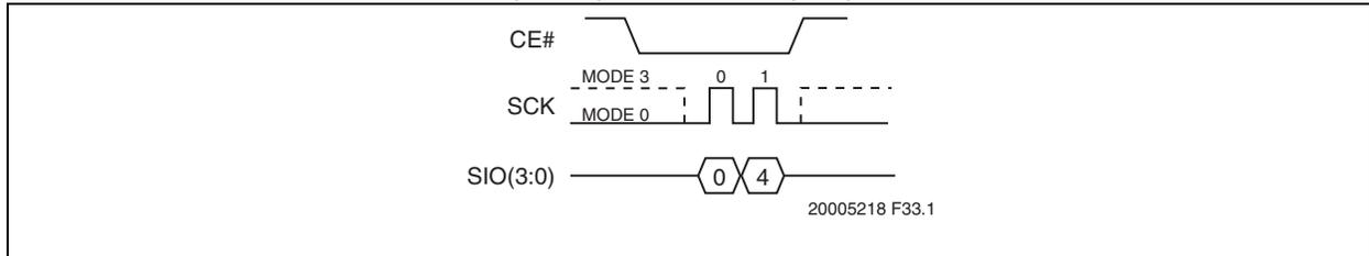
**FIGURE 5-35: WRITE-DISABLE (WRDI) SEQUENCE (SPI)**
