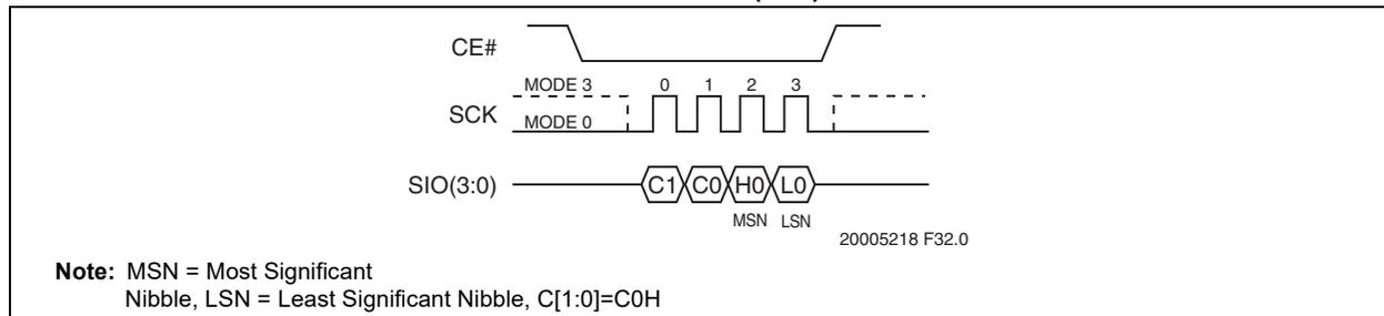
**FIGURE 5-12: SET BURST LENGTH SEQUENCE (SPI)**
