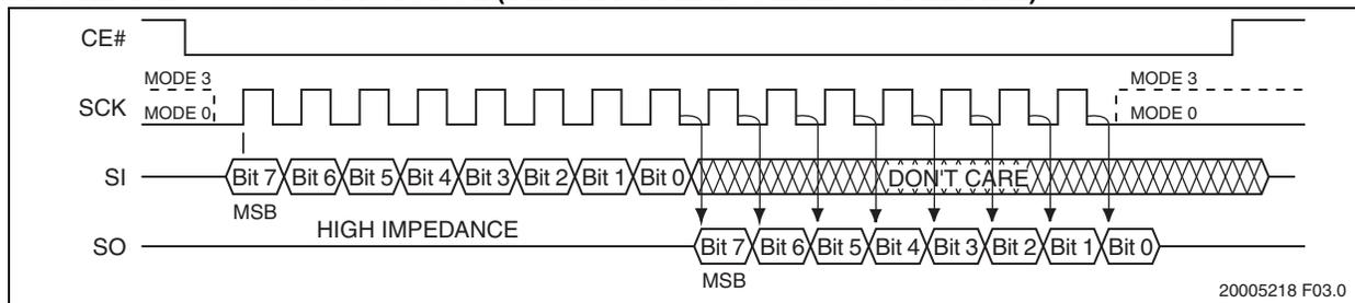
**FIGURE 4-2: SQI SERIAL QUAD I/O PROTOCOL**
