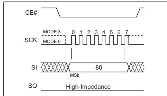
**FIGURE 5-6: AUTO ADDRESS INCREMENT (AAI) WORD PROGRAM SEQUENCE WITH HARDWARE END OF WRITE DETECTION**
