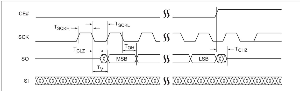
**FIGURE 8-3: HOLD TIMING DIAGRAM**
