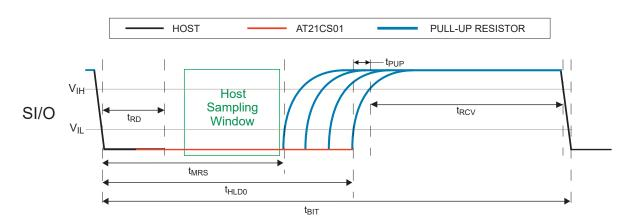
Figure 4-6. Logic '0' Data Output Bit Frame Waveform
