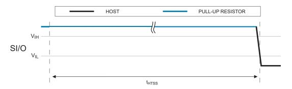
Figure 4-5. Stop Condition Waveform
