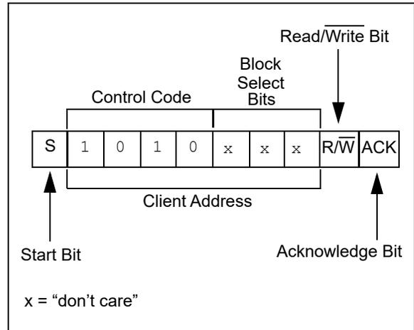
**FIGURE 5-2: ADDRESS SEQUENCE BIT ASSIGNMENTS**
