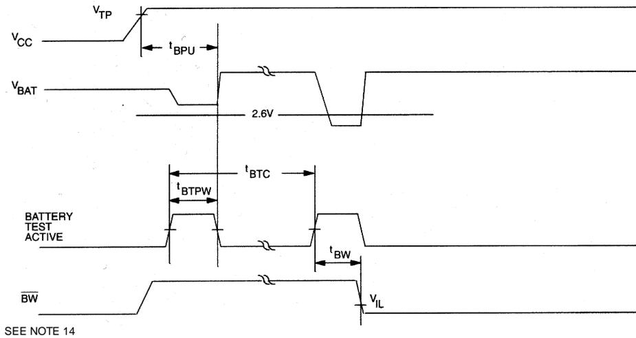
**POWER-DOWN/POWER-UP TIMING**(T<sub>A</sub>: See Note 10)
