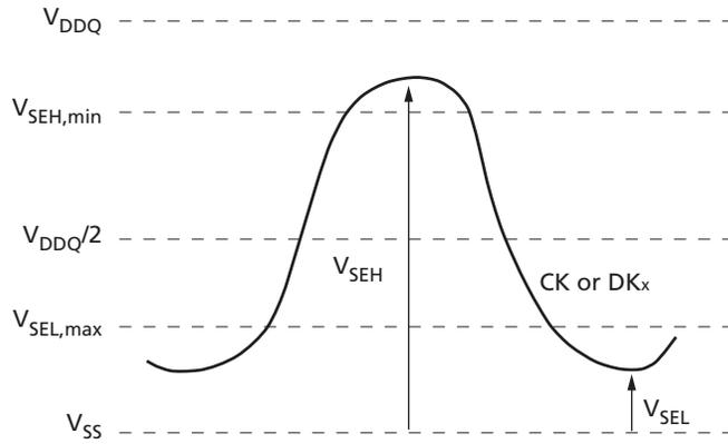
Figure 10: Definition of Differential AC Swing and  $t_{DVAC}$
