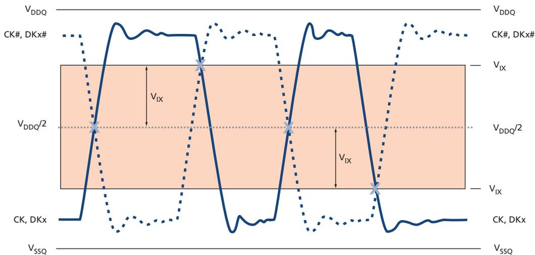
Figure 9: Single-Ended Requirements for Differential Signals
