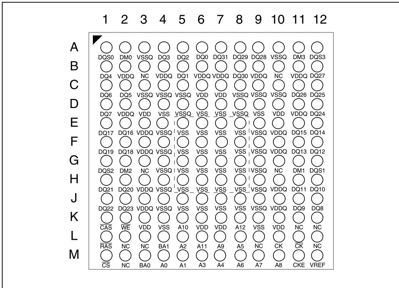
Note: Vss balls inside the dotted box are optional for purposes of thermal dissipation.
