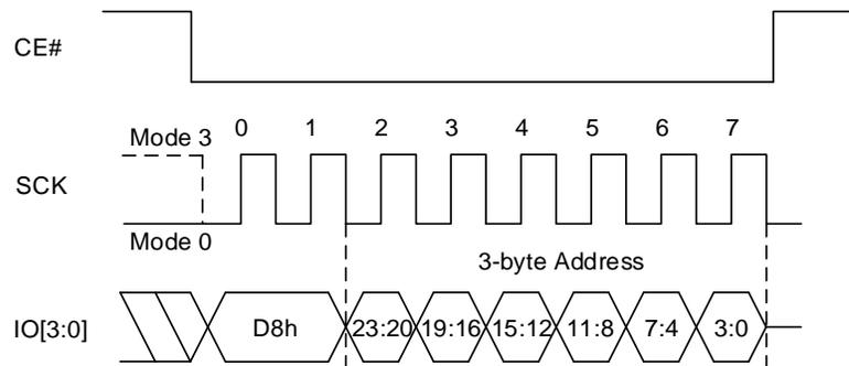
Figure 8.18 Block Erase (32K) Sequence In SPI Mode
