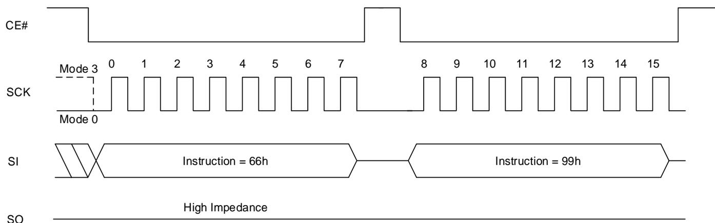
**Figure 8.59 Software Reset Enable and Software Reset Sequence In QPI Mode (RSTEN, 66h + RST, 99h)**
