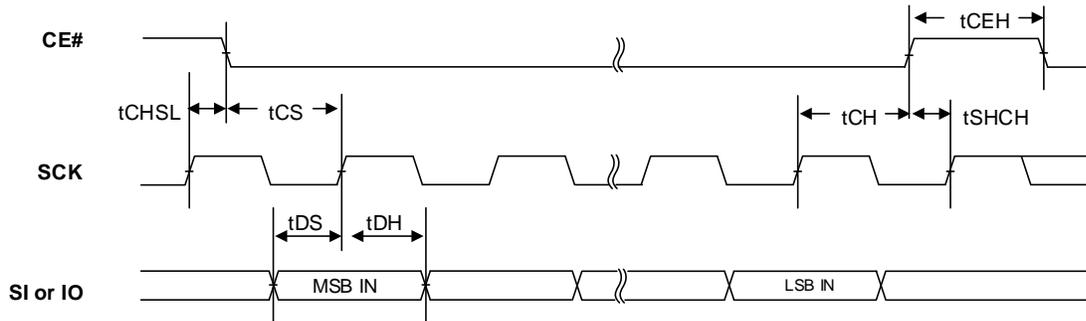
Figure 9.3 SERIAL INPUT TIMING (DTR Mode)
