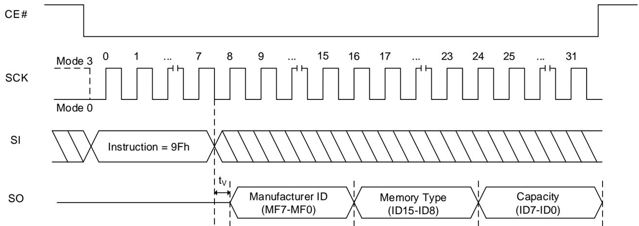
**Figure 8.53 RDJDID and RDJDIDQ (Read JEDEC ID) Sequence In QPI Mode**
