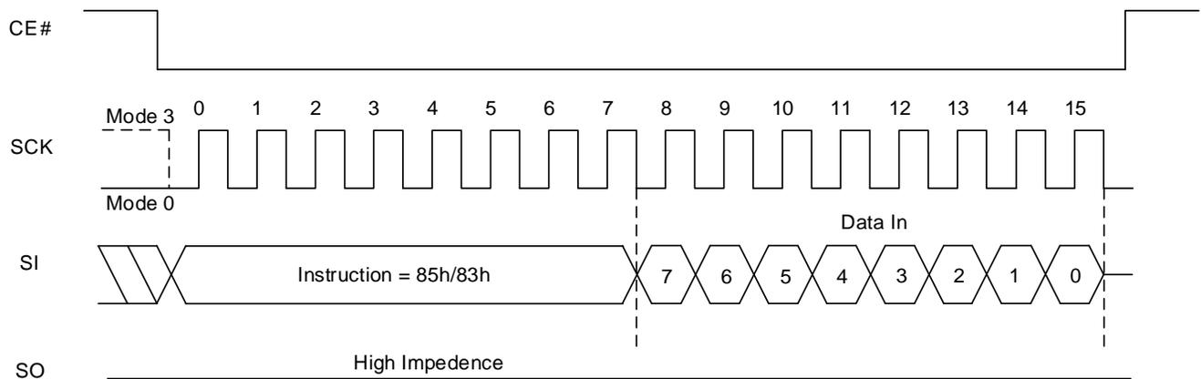
**Figure 8.43 Set Extended Read Parameters Sequence In QPI Mode**
