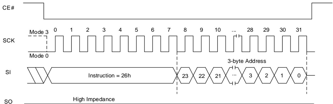
**Figure 8.71 Sector Unlock QPI Sequence In QPI Mode**
