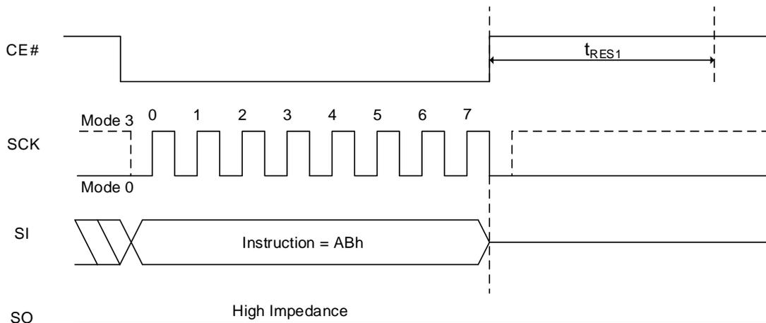
**Figure 8.39 Release Deep Power Down Mode Sequence In QPI Mode**
