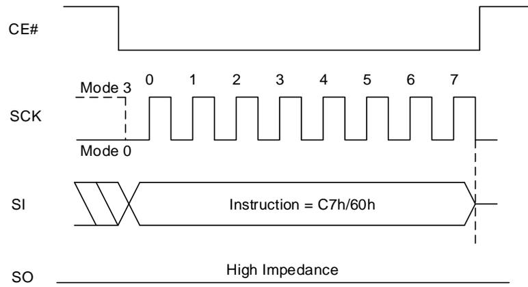
**Figure 8.21 Chip Erase Sequence In QPI Mode**
