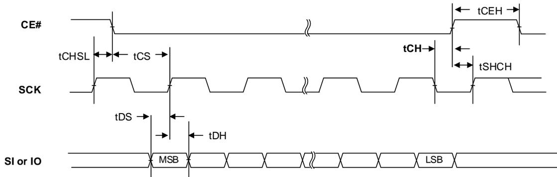
Figure 9.4 OUTPUT TIMING (STR Mode)
