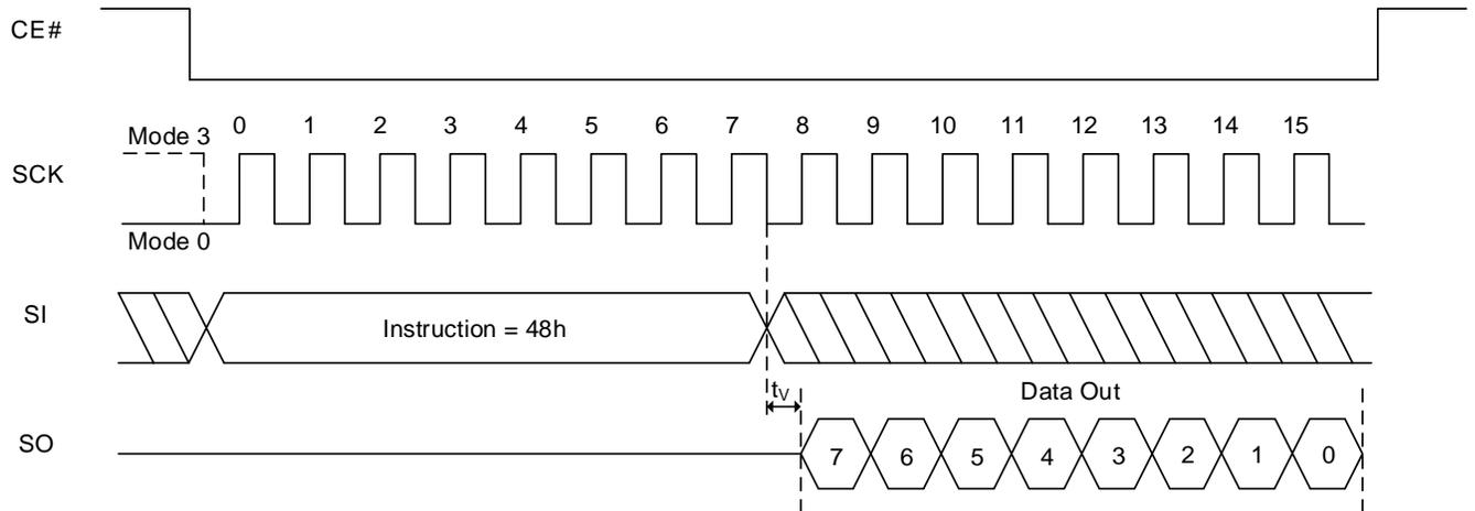
**Figure 8.31 Read Function Register Sequence In QPI Mode**
