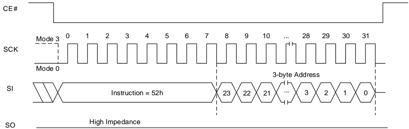
Figure 8.19 Block Erase (32K) Sequence In QPI Mode
