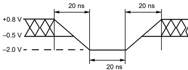
**Figure 9. Maximum Positive Overshoot Waveform**
