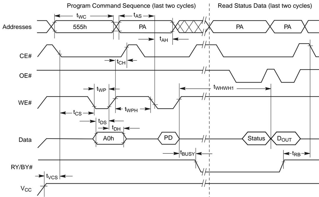
**Figure 17. Chip/Sector Erase Operation Timings<sup>[71, 72]</sup>**
