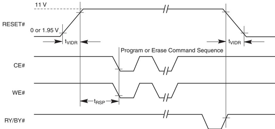
**Figure 22. Sector Group Protect/Unprotect Timing Diagram<sup>[77]</sup>**
