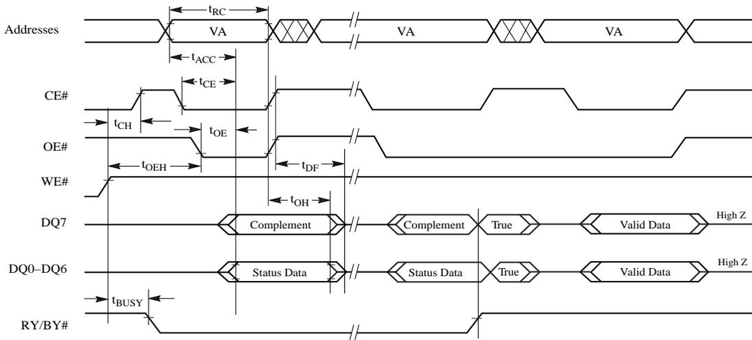
**Figure 19. Toggle Bit Timings (During Embedded Algorithms)<sup>[74]</sup>**
