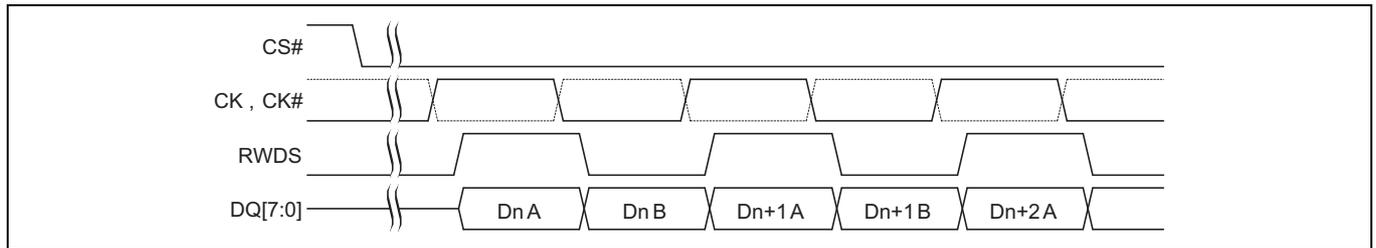
**Figure 4-2 Data Placement During a Read Transaction**<sup>[12, 13, 14, 15, 16]</sup>
