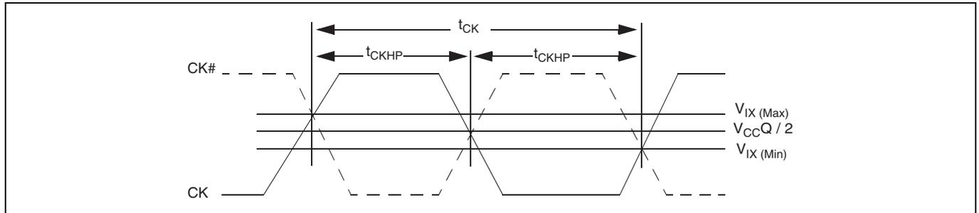
**Figure 10-3 Clock Characteristics**
