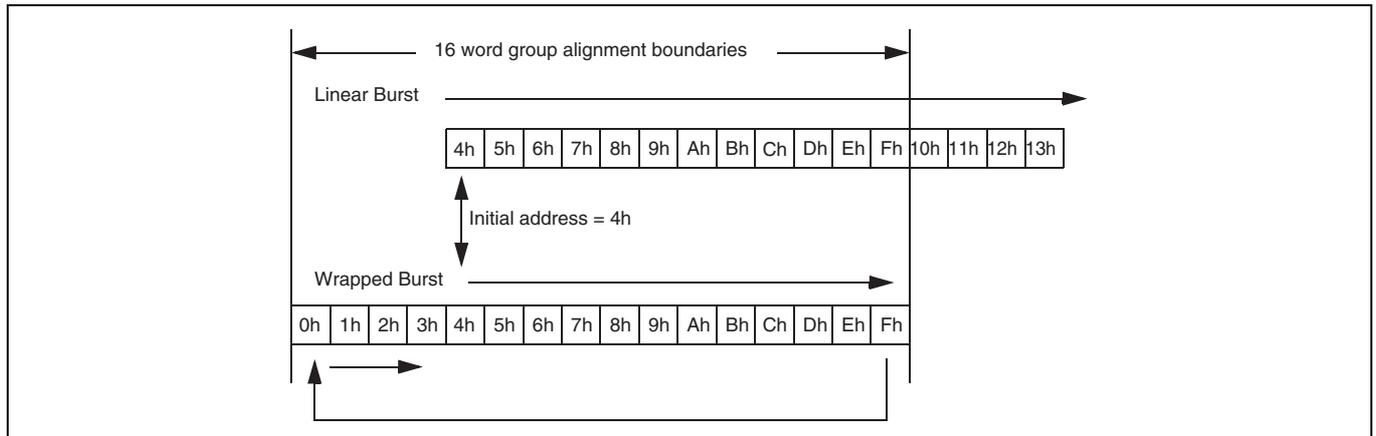
**Figure 1-4 Linear Versus Wrapped Burst Sequence**
