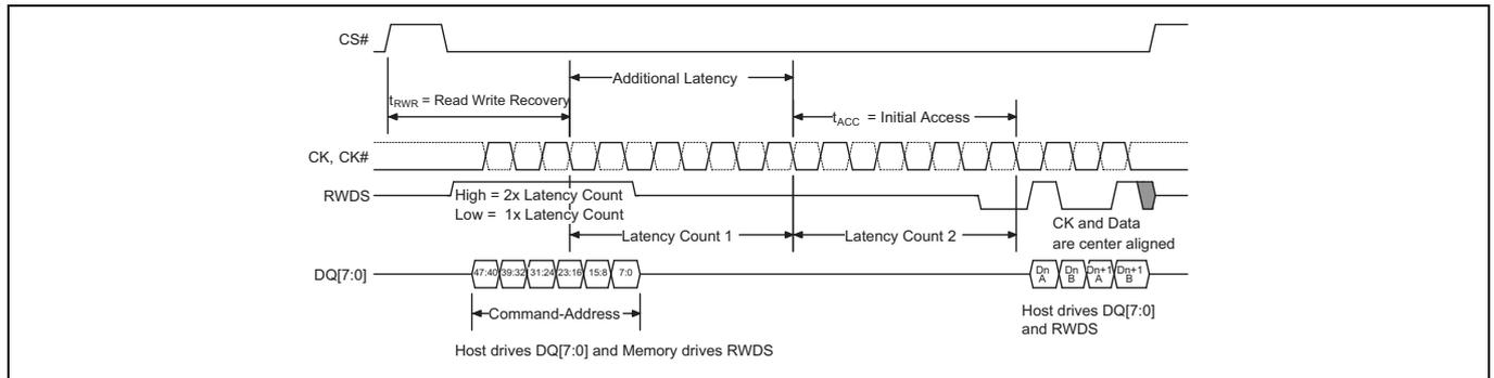
**Figure 4-6 Write Transaction with Additional Initial Latency**<sup>[30-36]</sup>
