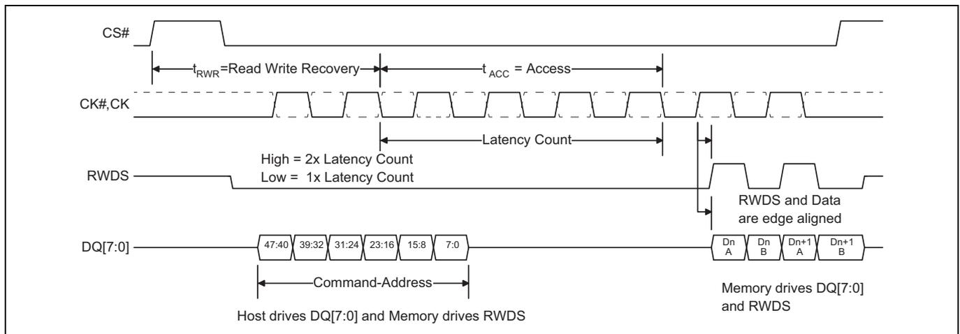
**Figure 1-1 Read Transaction, Single Initial Latency Count**
