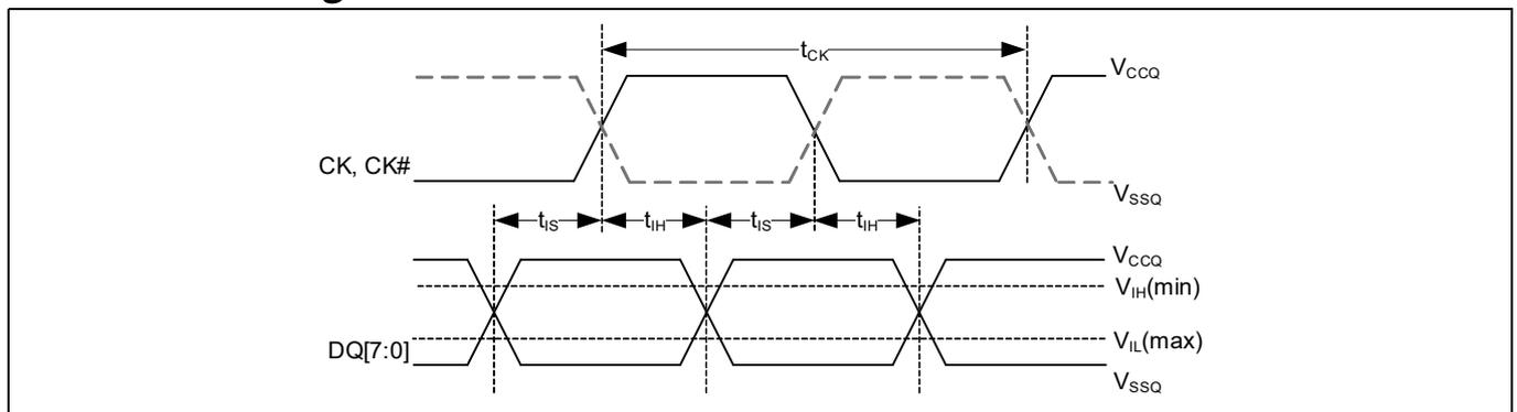
**Figure 10-8 DDR Input Timing Reference Levels**
