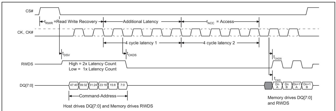
**Figure 10-6 Read Timing Diagram – With Additional Latency Required**
