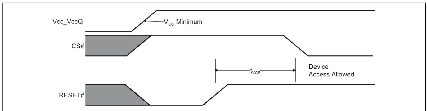
**Figure 9-4 Power-up with RESET# LOW**
