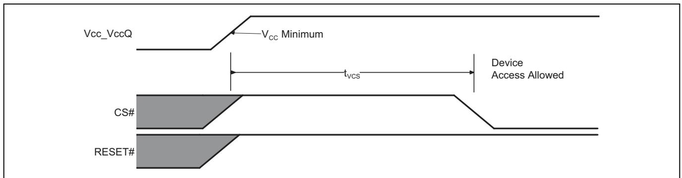
**Figure 9-3 Power-up with RESET# HIGH**
