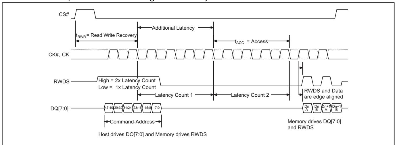
**Figure 4-4 Read Transaction with Additional Initial Latency**<sup>[21-28]</sup>
