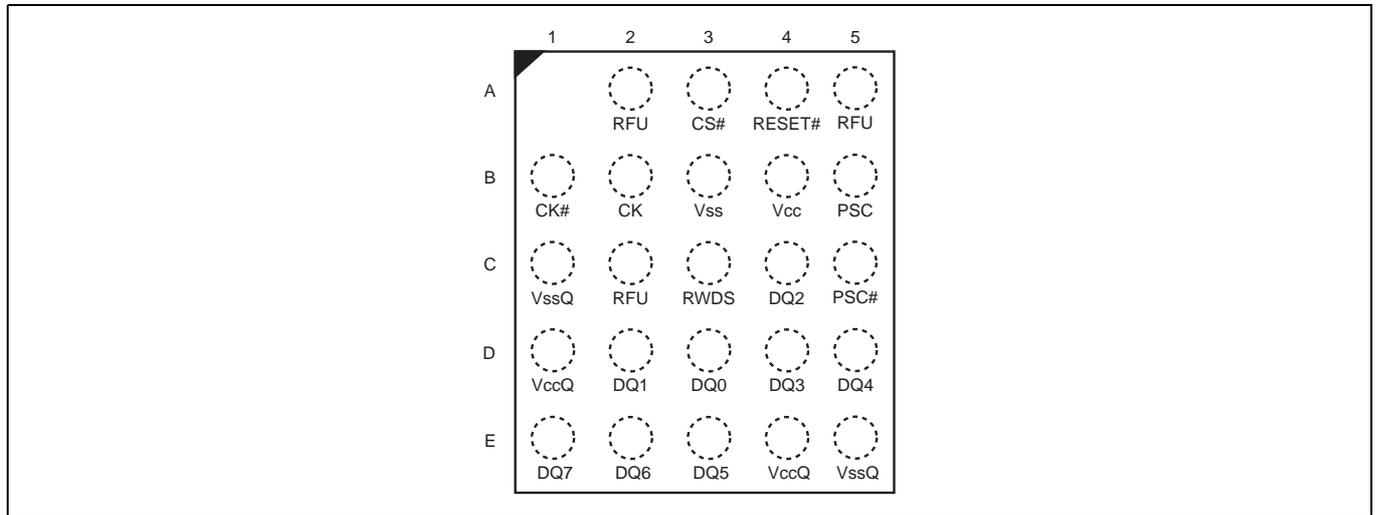
**Figure 12-2 24-ball FBGA, 5 × 5 Ball Footprint, Top View**
