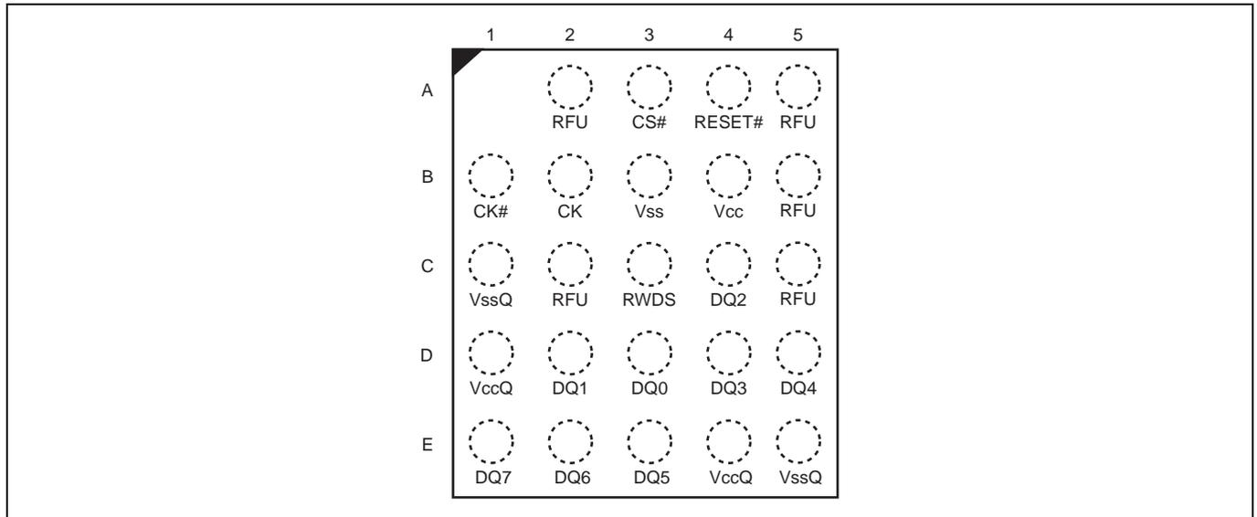
**Figure 11-1 24-Ball FBGA, 6 × 8 mm, 5 × 5 Ball Footprint, Top View**
