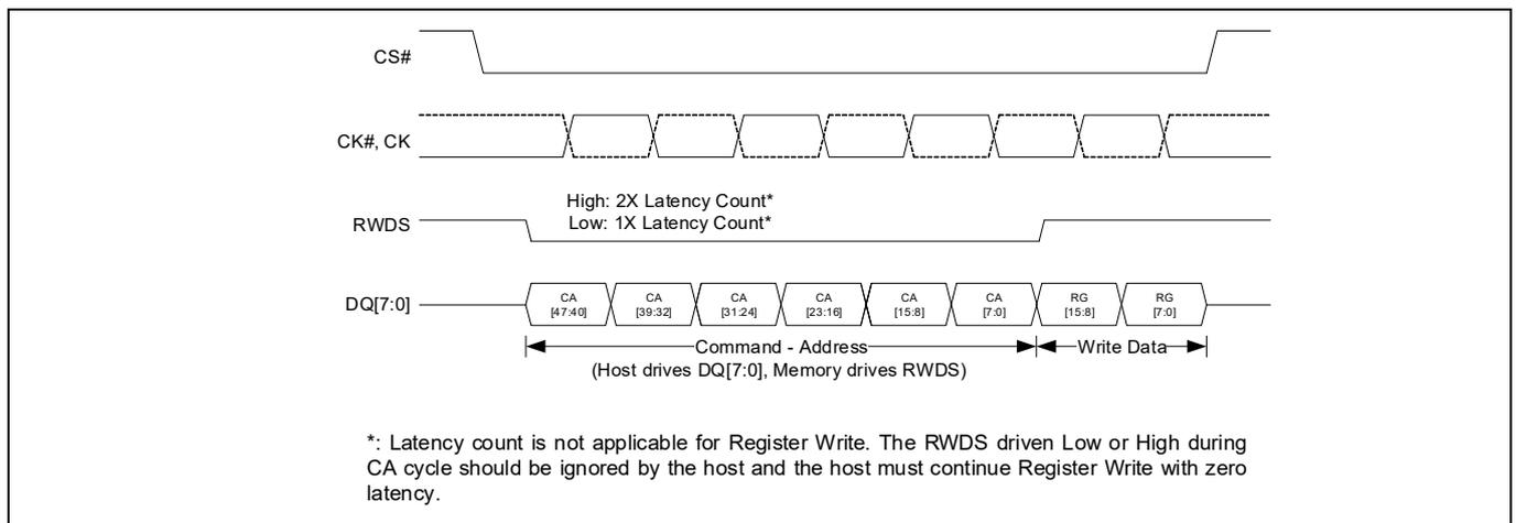
**Figure 4-8 Write Operation without Initial Latency**
