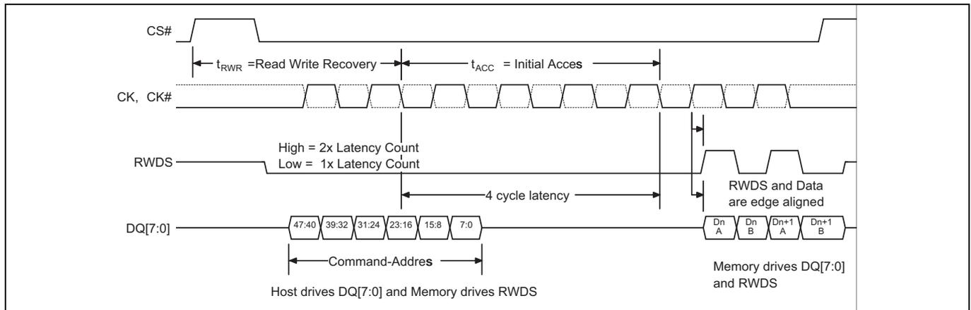
**Figure 4-5 Read Transaction Without Additional Initial Latency<sup>[29]</sup>**
