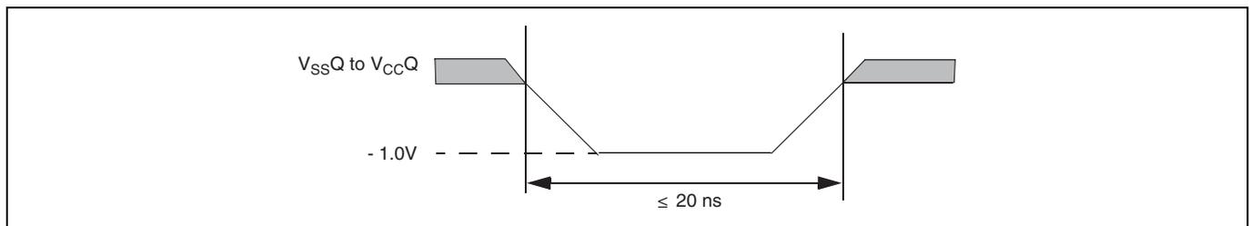
**Figure 9-1 Maximum Negative Overshoot Waveform**
