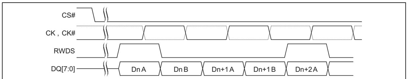
**Figure 4-3 Data Placement During a Write Transaction** <sup>[17, 18, 19, 20]</sup>
