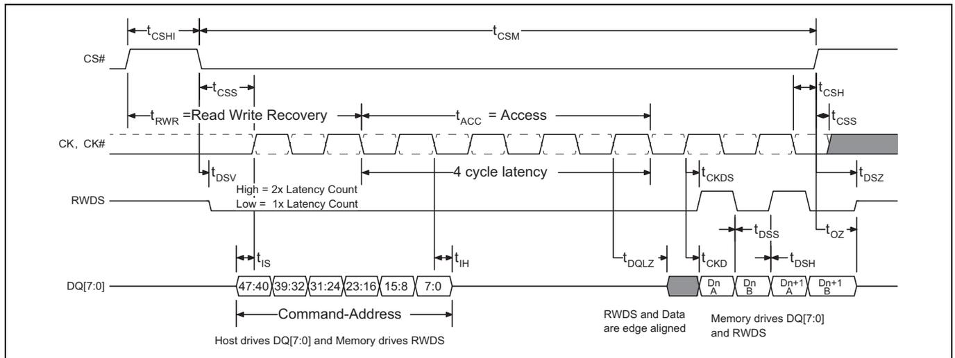
**Figure 10-5 Read Timing Diagram – No Additional Latency Required**
