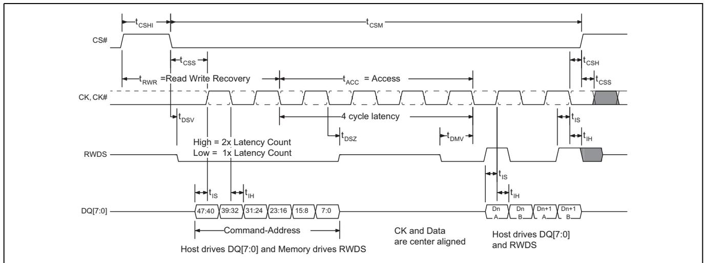
**Figure 10-7 Write Timing Diagram – No Additional Latency**
