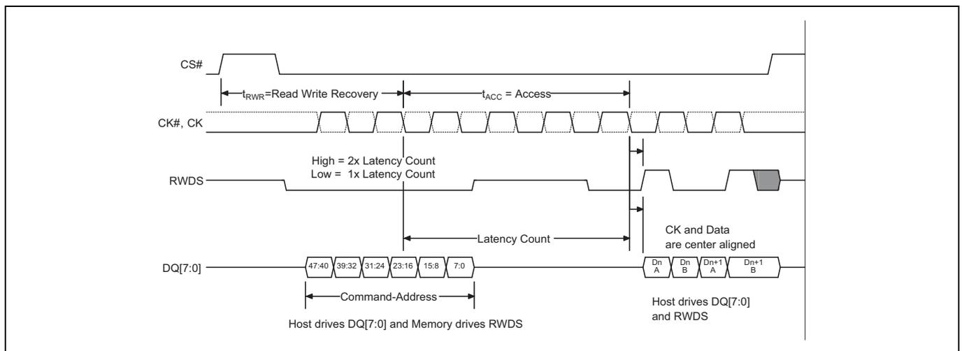
**Figure 4-7 Write Transaction Without Additional Initial Latency**<sup>[32-36]</sup>
