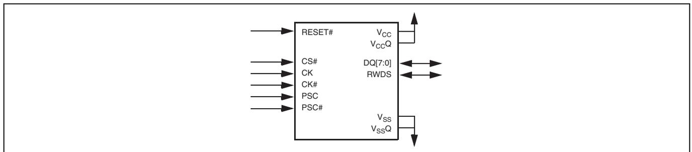
**Figure 12-1 HyperBus Product with DCARS Signal Diagram**
