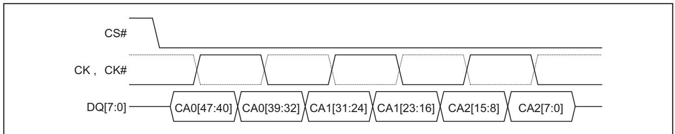
**Figure 4-1** Command-Address (CA) Sequence<sup>[4, 5, 6, 7]</sup>
