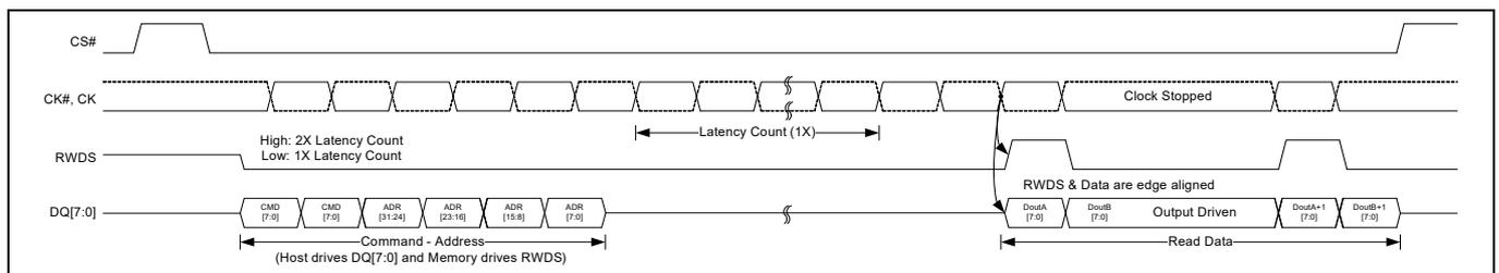
**Figure 8-1 Active Clock Stop During Read Transaction (DDR)<sup>[41]</sup>**
