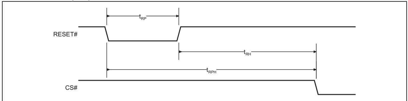
**Figure 9-6 Hardware Reset Timing Diagram**
