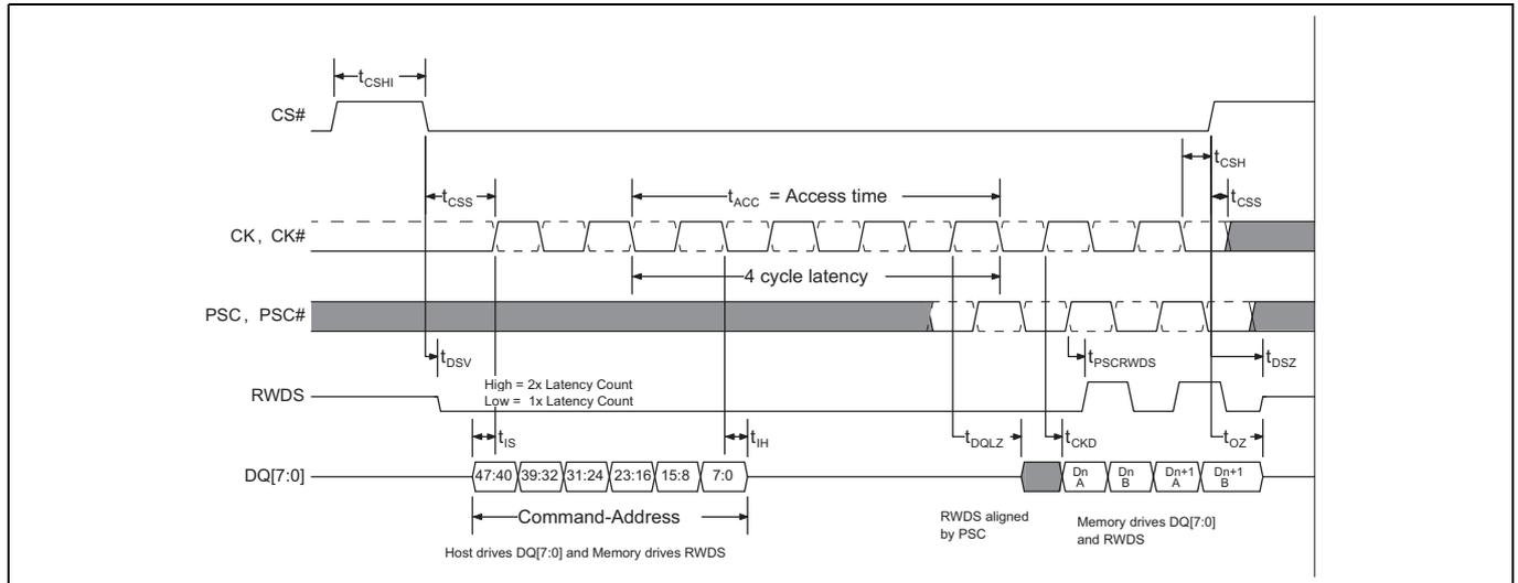
**Figure 12-3 HyperRAM Memory DCARS Timing Diagram** [65, 66, 67]
