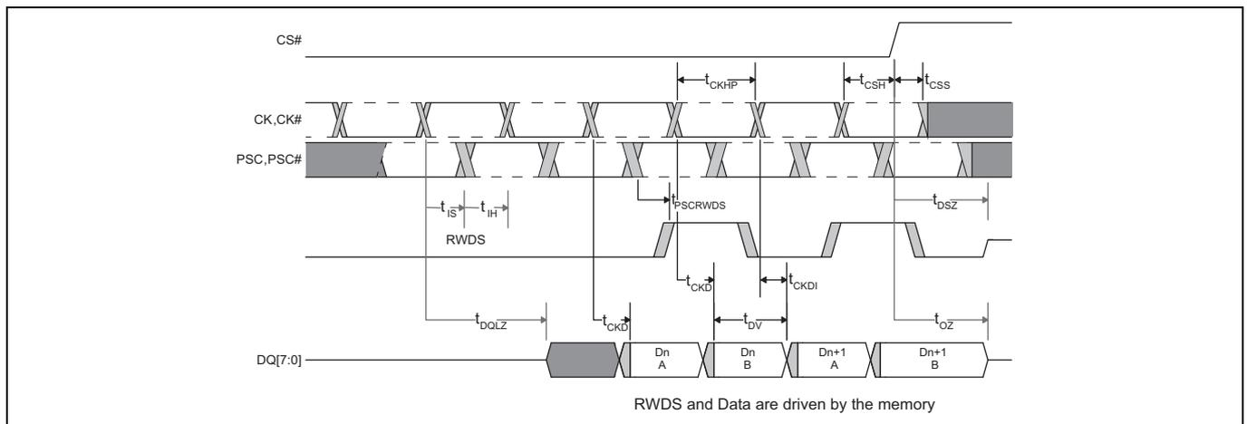
**Figure 12-4 DCARS Data Valid Timing** [72, 70, 70]
