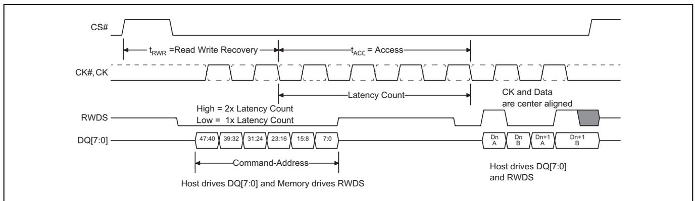
**Figure 1-3 Write Transaction, Single Initial Latency Count**
