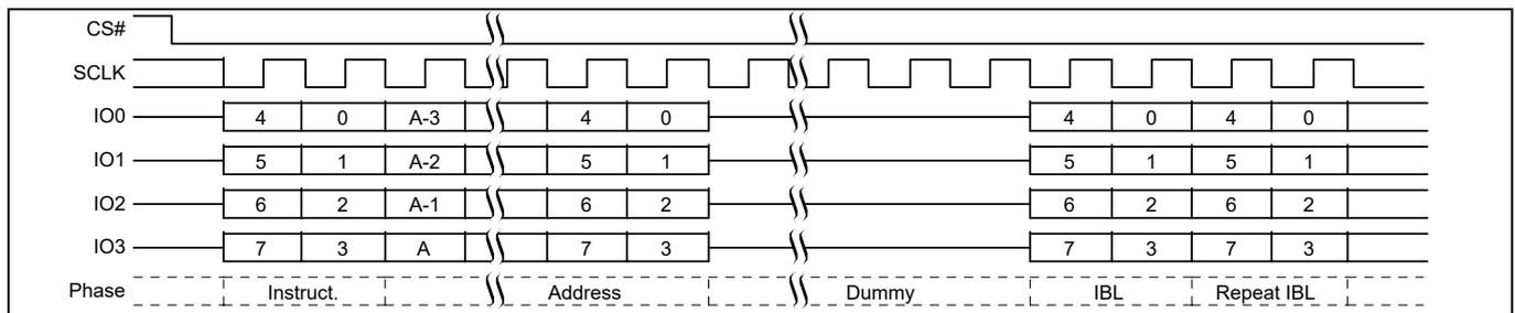
**Figure 96** IBLRD command sequence QPI<sup>[53, 54]</sup>
