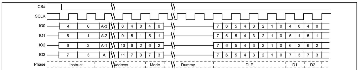
**Figure 75** DDR Quad I/O Read initial access QPI mode<sup>[40, 42]</sup>
