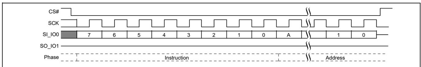
**Figure 82 Half Block Erase (HBE 52h or 4HBE 53h) command sequence**<sup>[47, 48]</sup>
