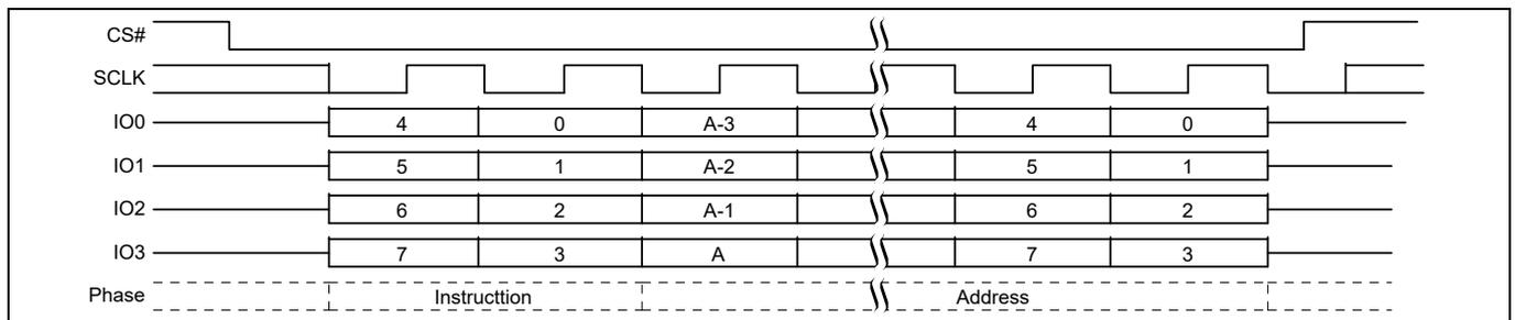
Figure 100 IBUL command sequence QPI mode<sup>[57, 58]</sup>
