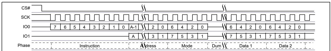
**Figure 69** Dual I/O Read command sequence<sup>[36, 37]</sup>
