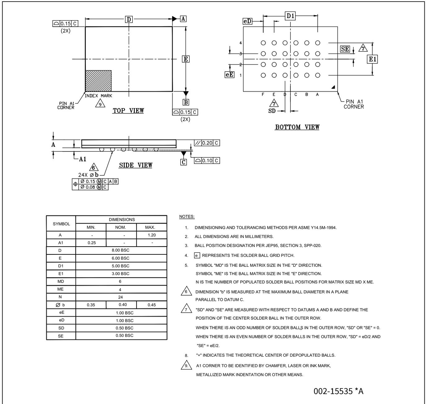
Figure 155 24-ball FBGA (8 × 6 × 1.2 mm) package outline (PG-TFBGA-24), 002-15535
