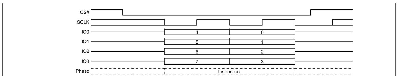
**Figure 87** Chip Erase command sequence QPI mode
