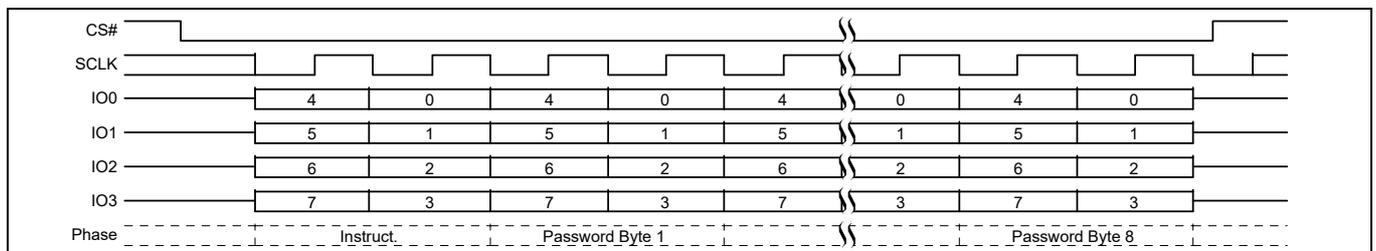
**Figure 120 Password Unlock (PASSU) command sequence QPI mode**
