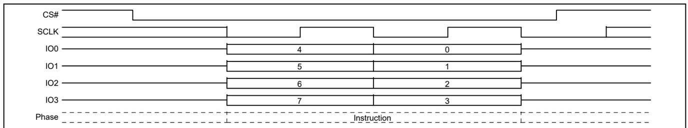
**Figure 114 Protection Register Lock (PRL) command sequence – QPI mode**
