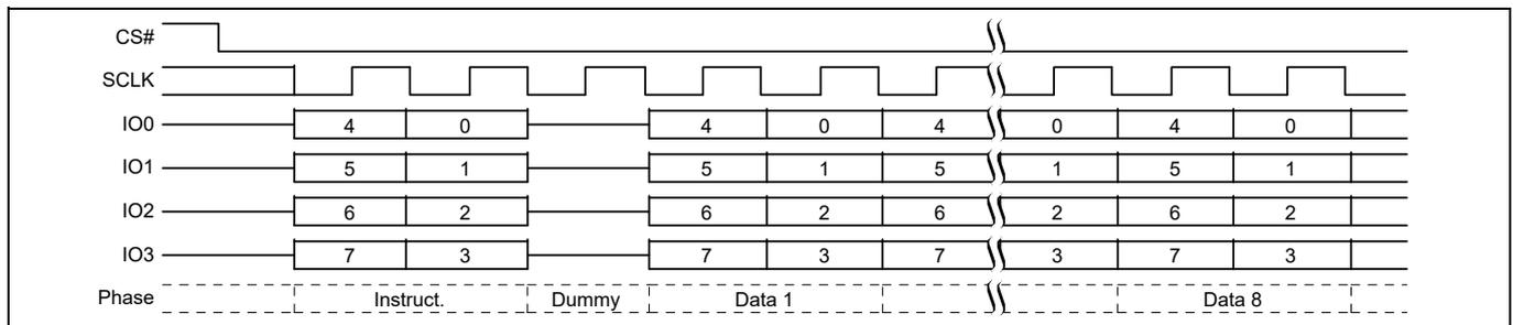
**Figure 116 Password Read (PASSRD) command sequence – QPI mode**
