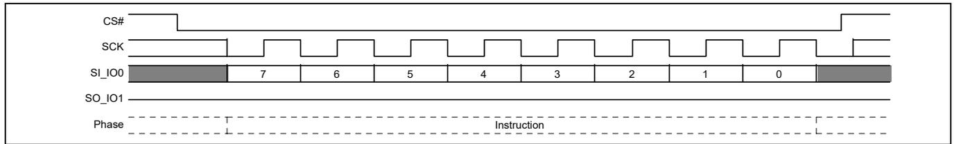
**Figure 88** Program or Erase Suspend command sequence
