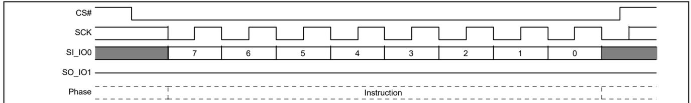
**Figure 63** Enter QPI Mode (QPIEN 38h) command sequence
