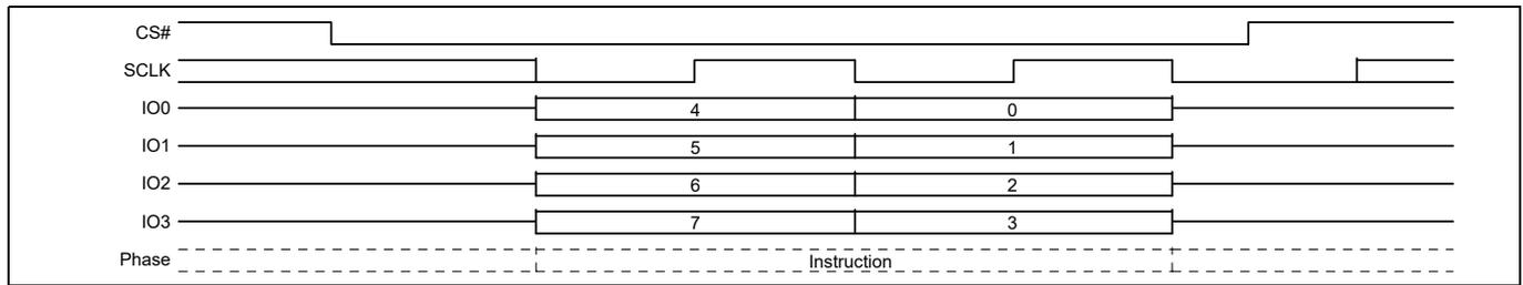
**Figure 44 Write Disable (WRDI) command sequence QPI mode**
