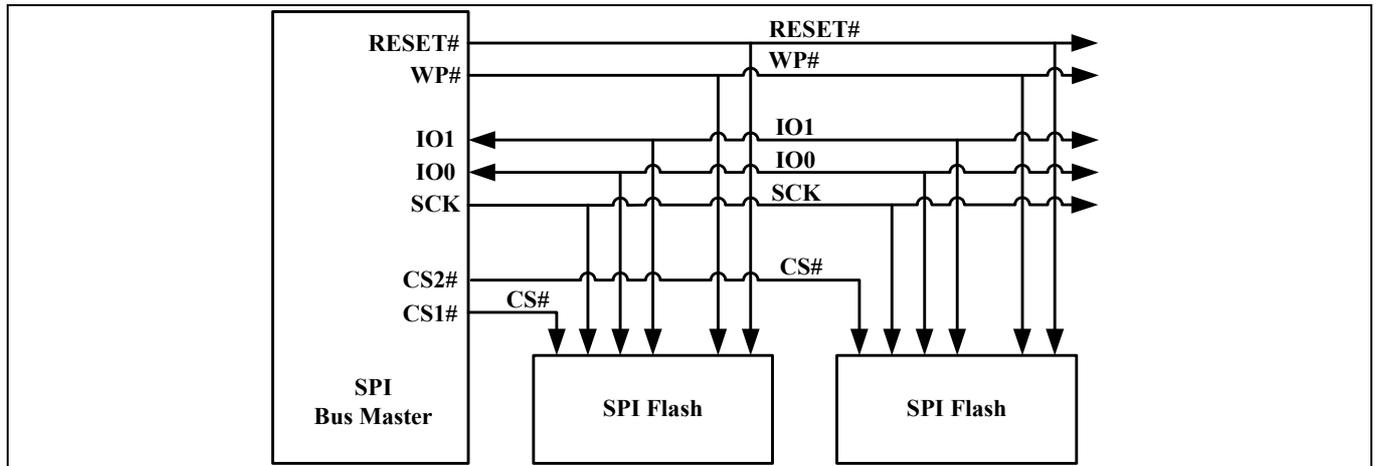
Figure 8 Bus master and memory devices on the SPI bus - dual bit data path
