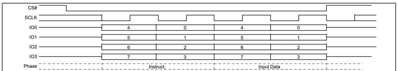
**Figure 52 Write DLRV (WDLRV) command sequence – QPI mode**
