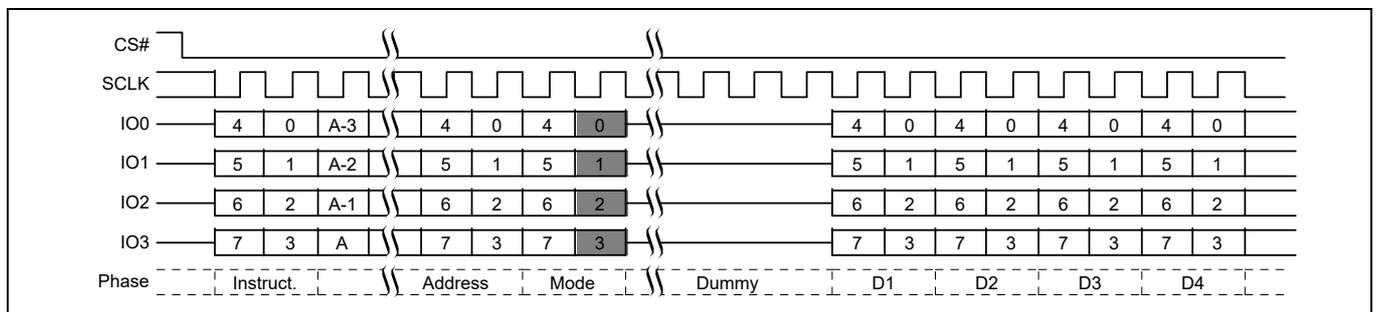
Figure 72 Quad I/O Read initial access command sequence QPI mode<sup>[38]</sup>
