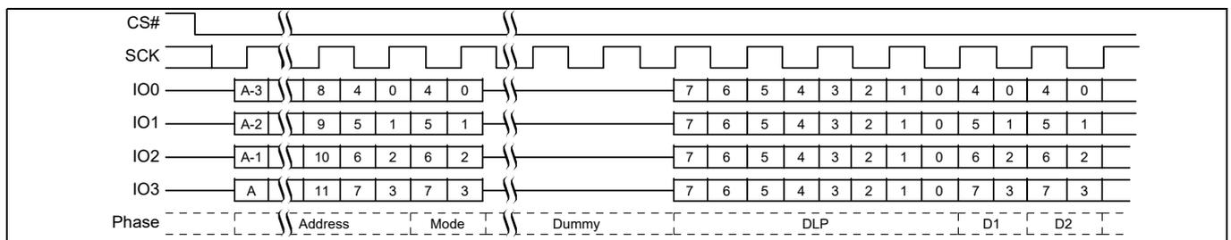
**Figure 76** Continuous DDR Quad I/O Read subsequent access<sup>[40, 41, 42]</sup>
