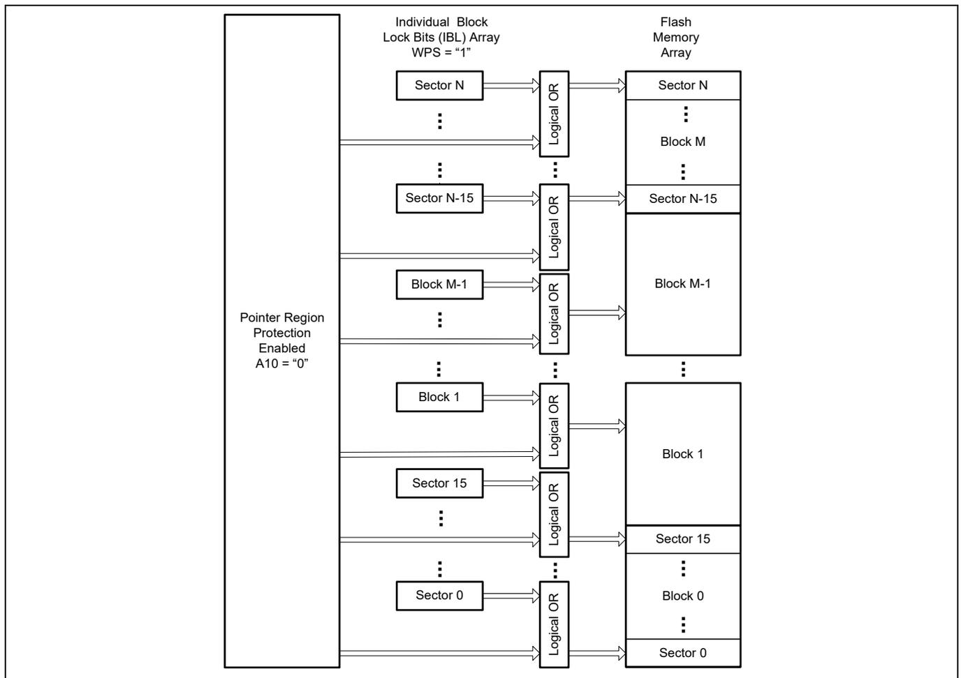
Figure 25 Individual block lock / pointer region protection control
