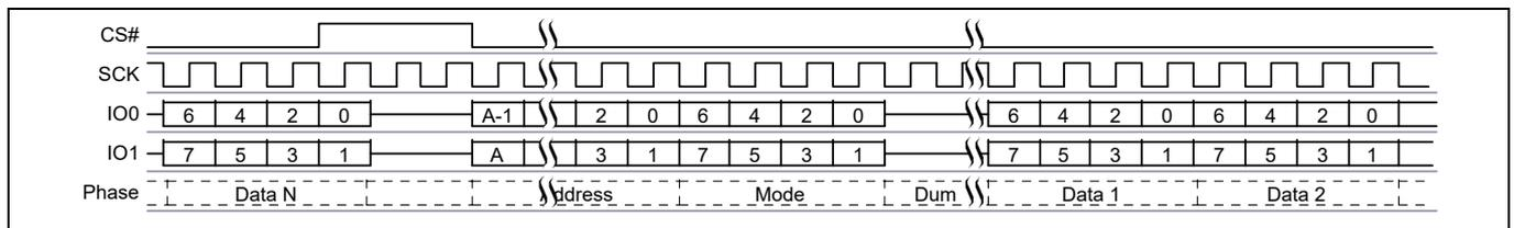
**Figure 70** Dual I/O Continuous Read command sequence<sup>[36]</sup>
