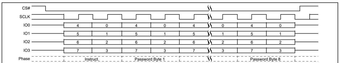
**Figure 118 Password Program (PASSP) command sequence QPI mode**
