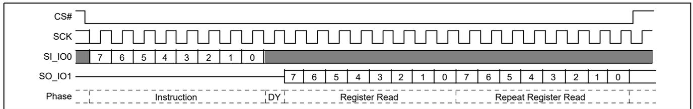
**Figure 111 Protection Register Read (PRRD) command sequence**
