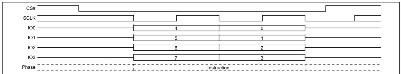
**Figure 42 Write Enable (WREN) command sequence QPI mode**
