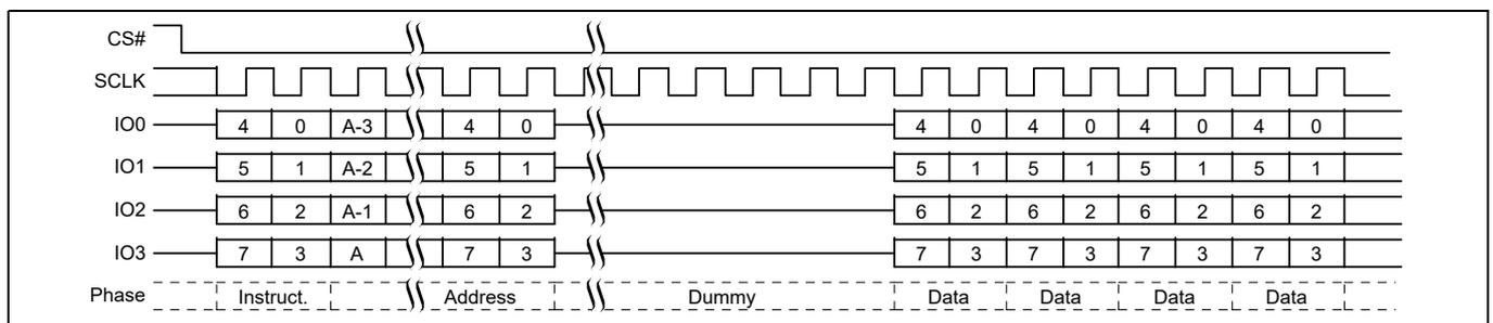
**Figure 60** Read Any Register, QPI mode, command sequence<sup>[31]</sup>
