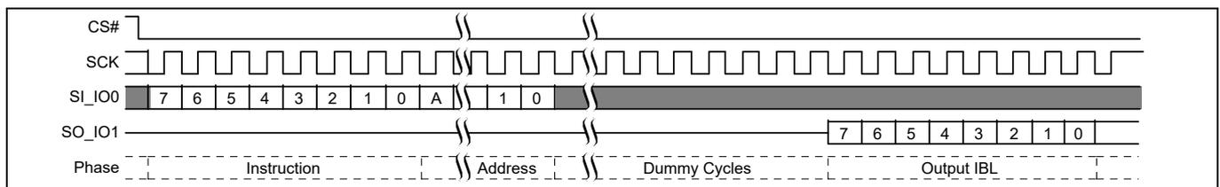
**Figure 95** IBLRD command sequence<sup>[53, 54]</sup>
