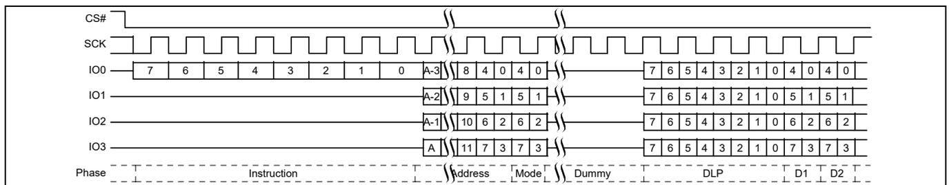
**Figure 74** DDR Quad I/O Read initial access<sup>[40, 42]</sup>
