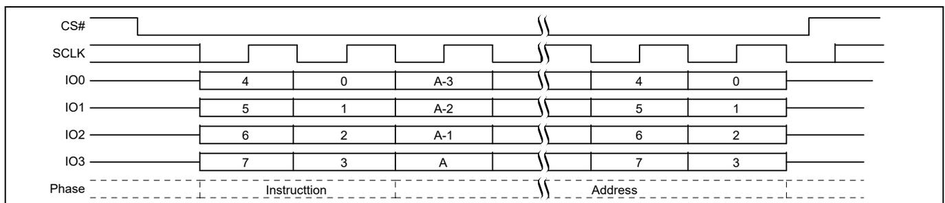
**Figure 85** Block Erase (BE D8h or 4BE DCh) QPI mode command sequence<sup>[49]</sup>
