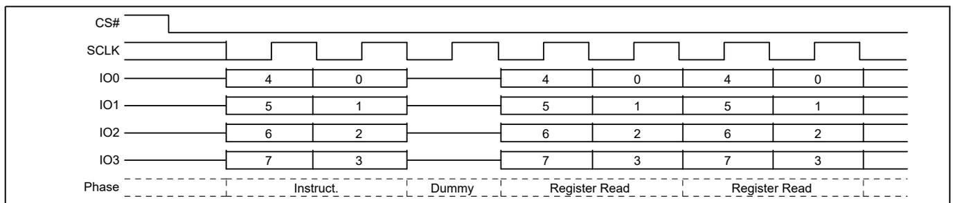
**Figure 54 DLP Read (DLPRD) command sequence – QPI mode**
