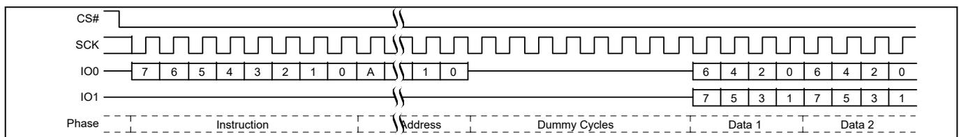
**Figure 67** Dual Output Read command sequence<sup>[34]</sup>
