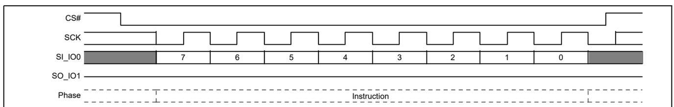
Figure 123 Deep Power Down (DPD) command sequence
