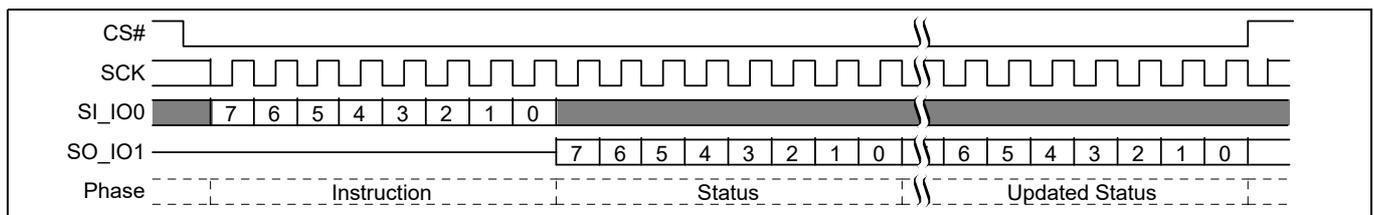
**Figure 37** Read Status Register 2 (RDSR2) Command
