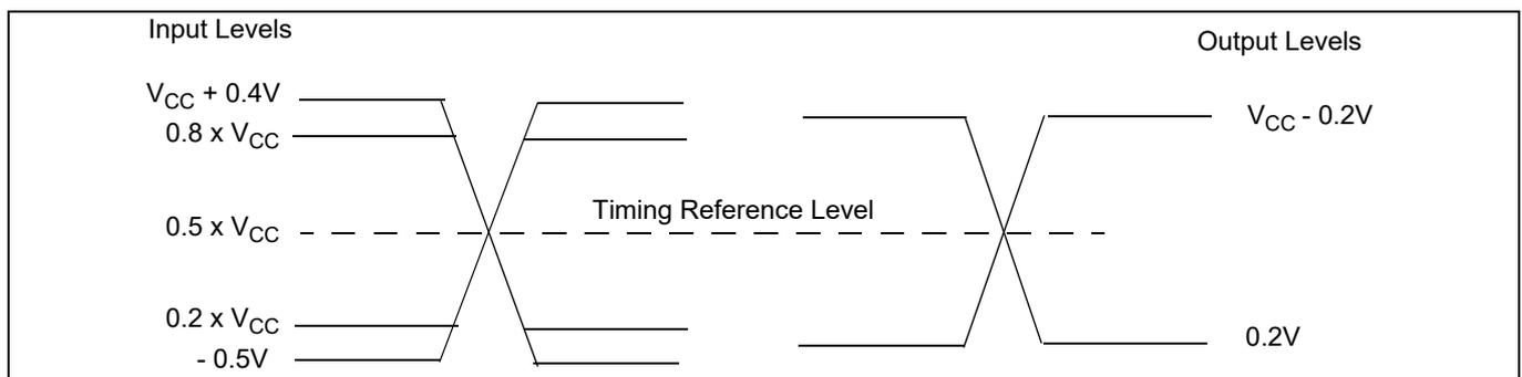
Figure 135 Input, output, and timing reference levels
