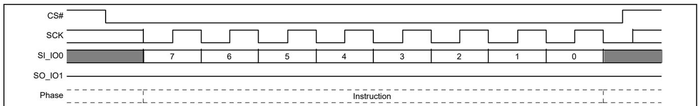
**Figure 121 Software / Mode Bit Reset command sequence**
