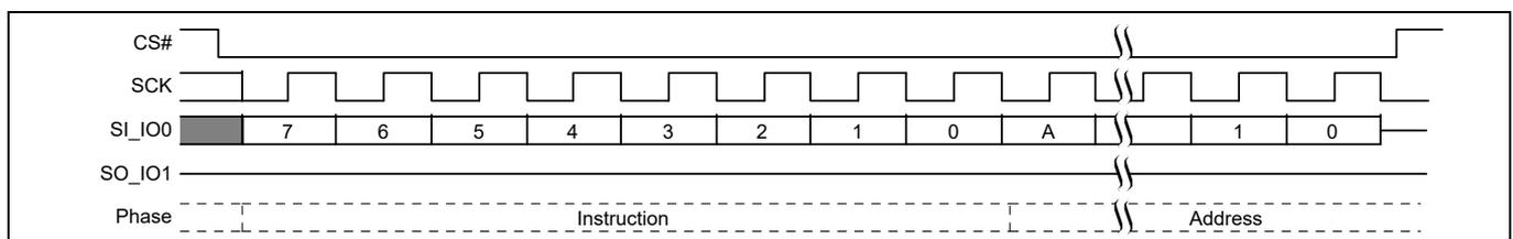
**Figure 80** Sector Erase (SE 20h or 4SE 21h) command sequence<sup>[46]</sup>
