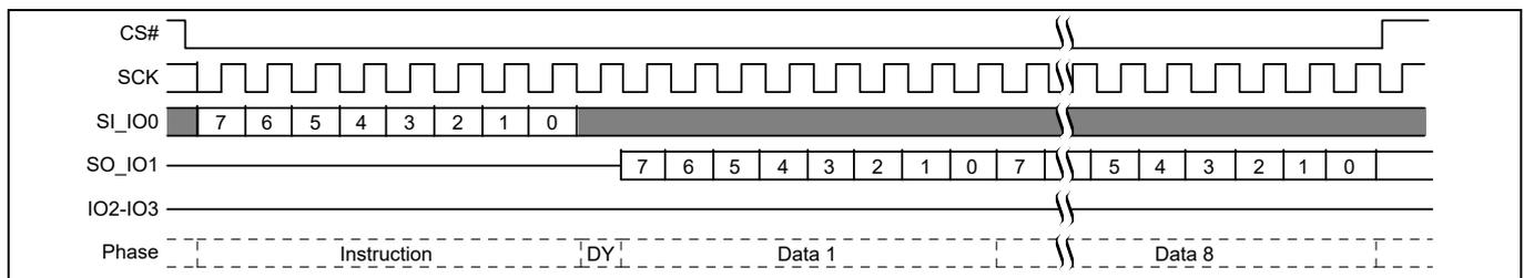
**Figure 115 Password Read (PASSRD) command sequence**
