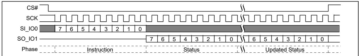
**Figure 35** Read Status Register 1 (RDSR1) command sequence
