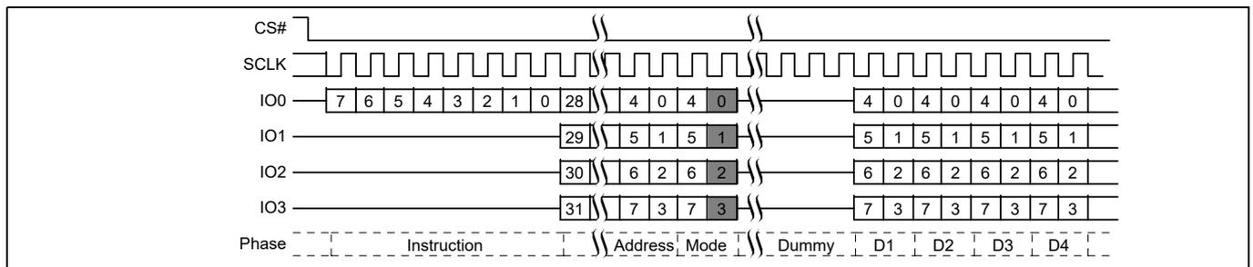
Figure 20 Quad I/O command<sup>[8]</sup>
