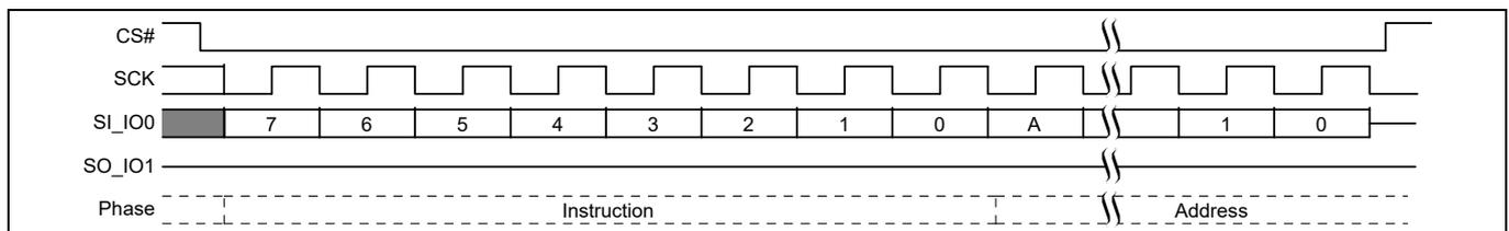
**Figure 84** Block Erase (BE D8h or 4BE DCh) command sequence<sup>[49]</sup>
