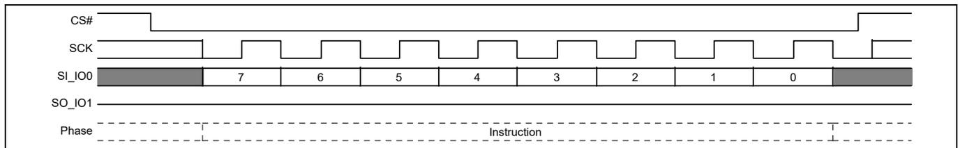
**Figure 113 Protection Register Lock (PRL) command sequence**
