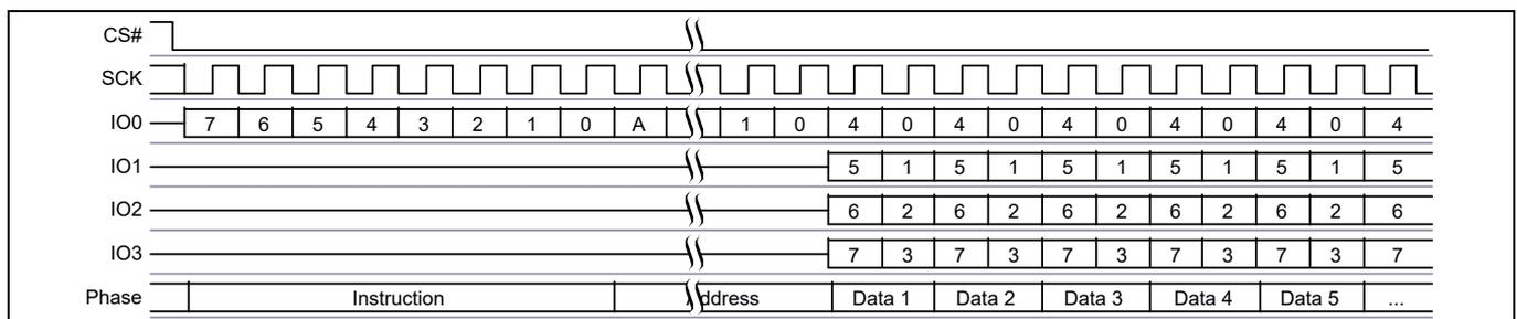
**Figure 79** Quad page program command sequence<sup>[45]</sup>
