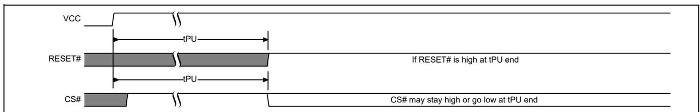
Figure 137 Reset high at the end of POR
