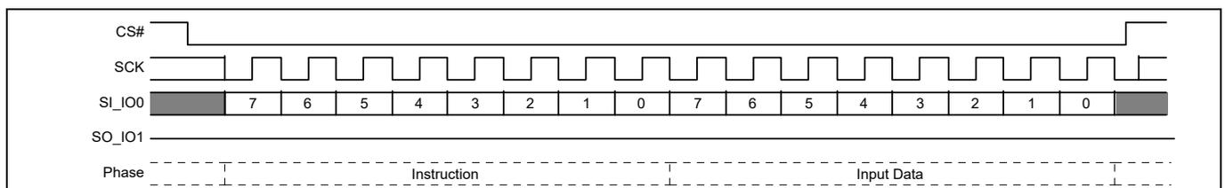
**Figure 49 Program DLRNV (PDLRNV) command sequence**
