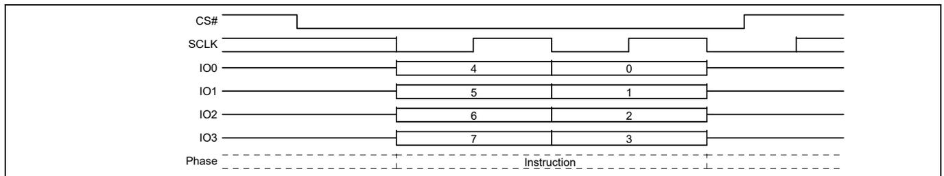
**Figure 89** Program or Erase Suspend command sequence QPI mode
