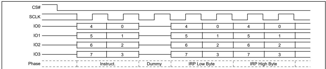
Figure 108 IRPRD command sequence – QPI mode
