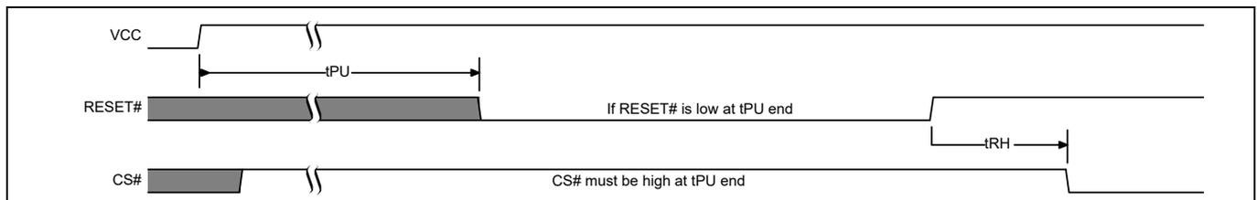
Figure 136 Reset low at the end of POR
