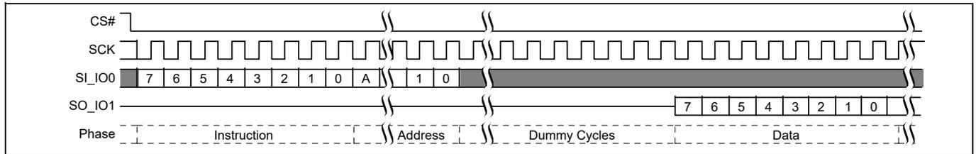
**Figure 59** Read Any Register Read command sequence<sup>[31]</sup>
