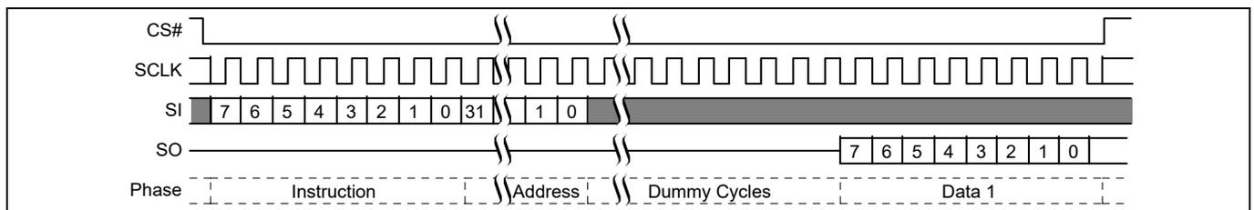
**Figure 16 Single Bit Wide I/O command with latency**
