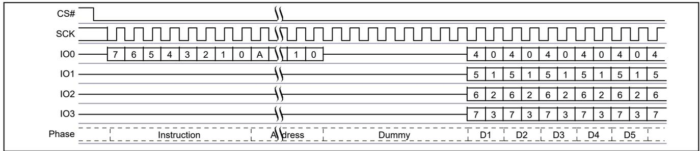
**Figure 68 Quad Output Read command sequence<sup>[35]</sup>**
