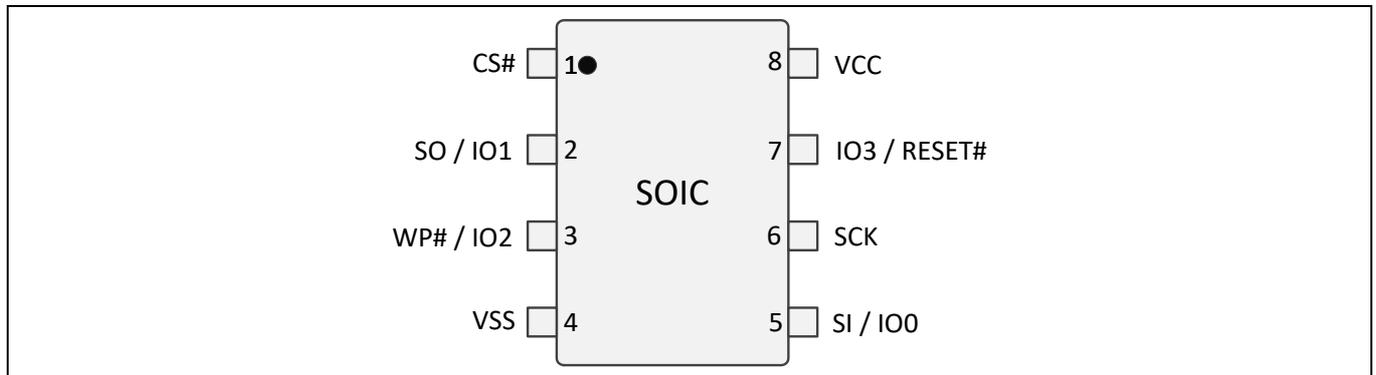
Figure 2 8-Pin plastic small outline package (SOIC8)
