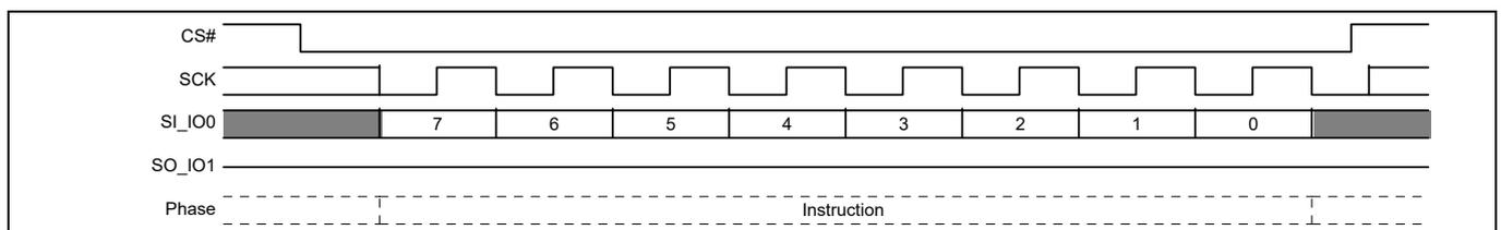
**Figure 55 Enter 4 Byte Address Mode (4BEN B7h) command sequence**
