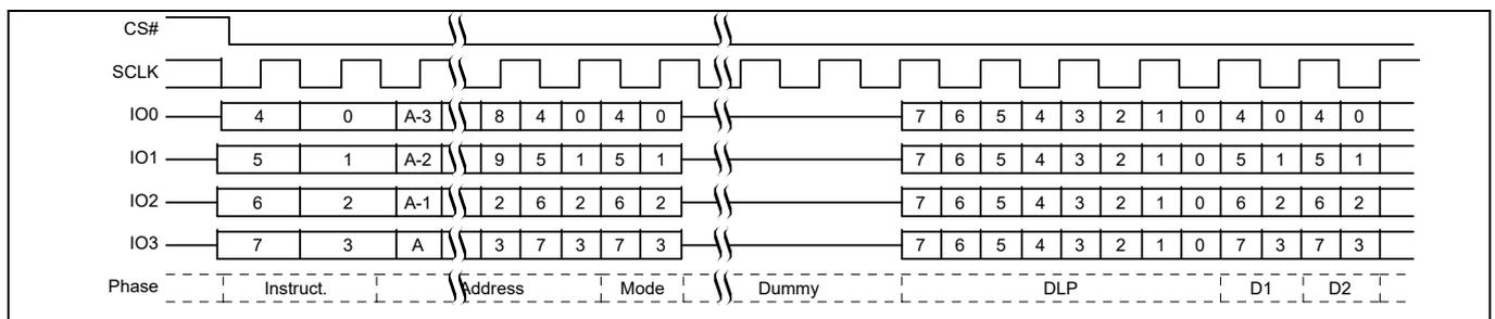
Figure 23 DDR Quad I/O Read command QPI mode
