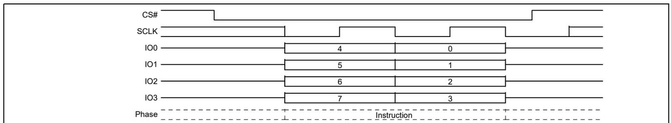
**Figure 64** Exit QPI (QPIEX F5h) command sequence
