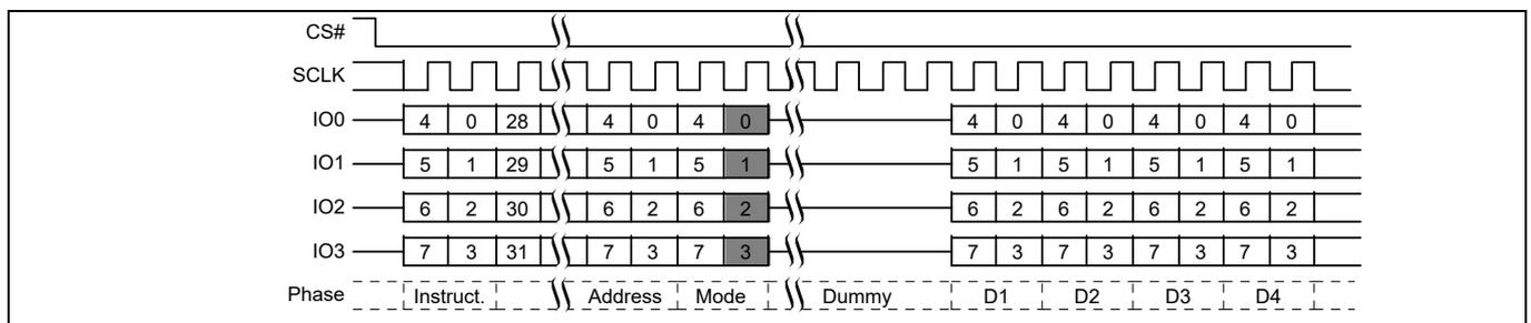
Figure 21 Quad I/O Read command in QPI mode<sup>[8]</sup>
