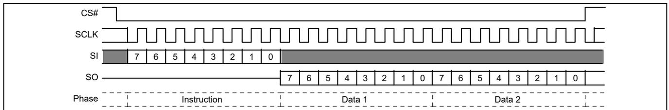
**Figure 15 Single Bit Wide Output command without latency**
