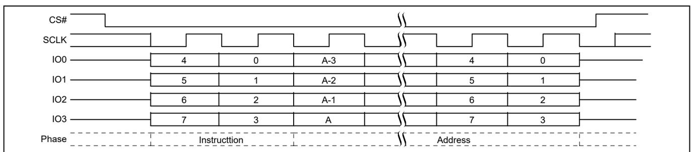
**Figure 81** Sector Erase (SE 20h or 4SE 21h) QPI mode command sequence<sup>[46]</sup>
