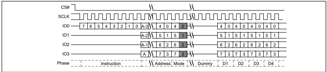
Figure 71 Quad I/O Read initial access command sequence<sup>[38]</sup>
