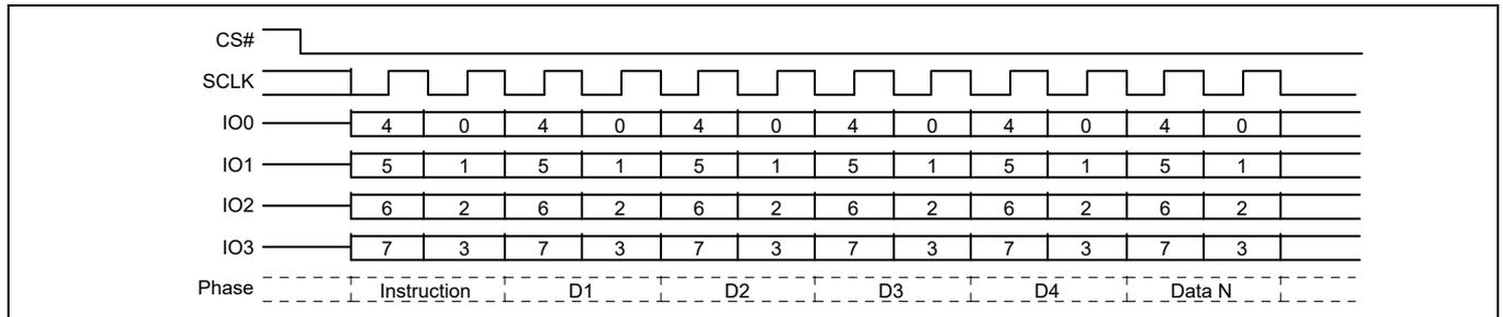
**Figure 28 Read Identification (RDID) QPI mode command**
