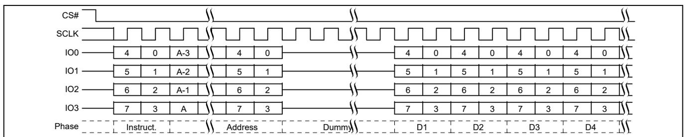
**Figure 94 Security Regions Read command sequence QPI mode**<sup>[52]</sup>
