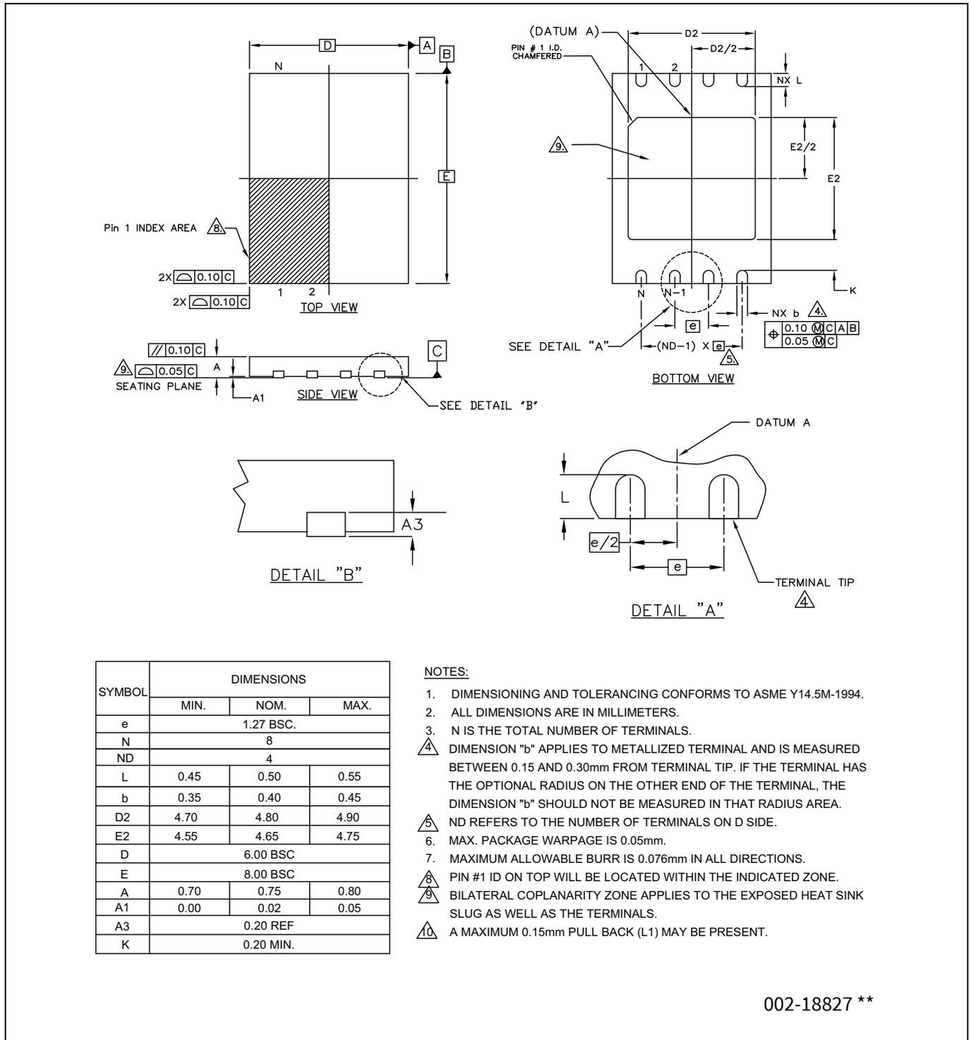
Figure 153 8-lead DFN ((6 x 8 x 0.8 mm) 4.80 x 4.65 mm E-Pad (Sawn)) package outline (PG-WSO8-8), 002-18827
