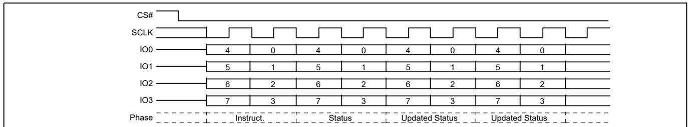
**Figure 36** Read Status Register 1 (RDSR1) QPI Mode Command
