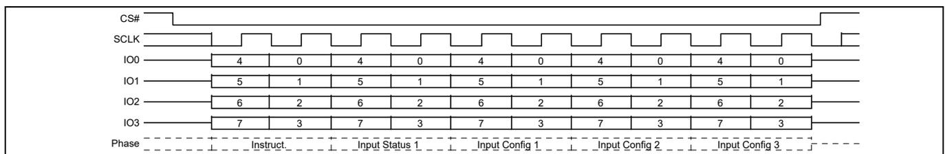
**Figure 40 Write Register (WRR) command sequence QPI mode**
