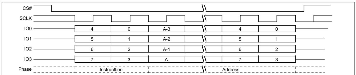
Figure 98 IBL command sequence QPI mode<sup>[55, 56]</sup>
