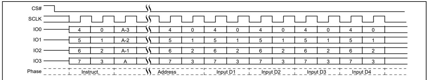
**Figure 78** Page Program (PP 02h or 4PP 12h) QPI mode command sequence<sup>[44]</sup>
