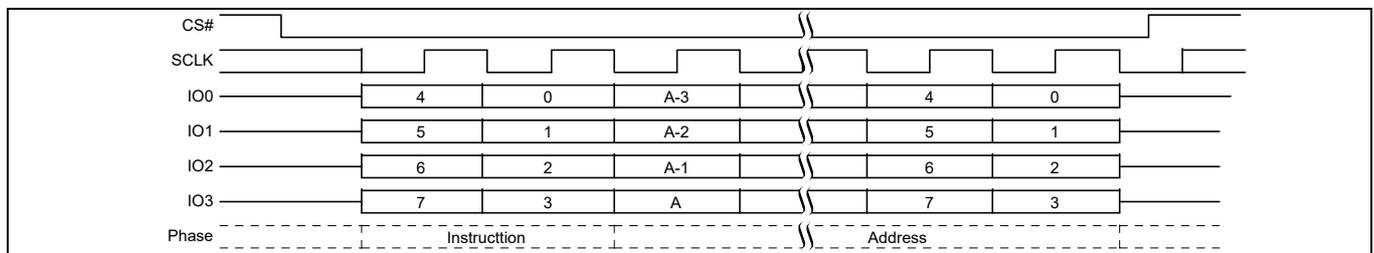
Figure 106 SPRP command sequence QPI mode<sup>[59, 60]</sup>
