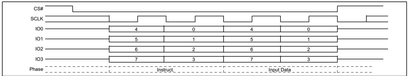
**Figure 50 Program DLRNV (PDLRV) command sequence – QPI mode**
