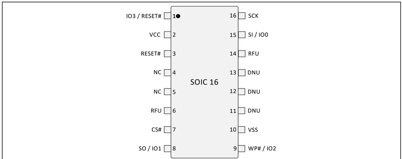
Figure 1 16-lead SOIC package (SO3016), top view
