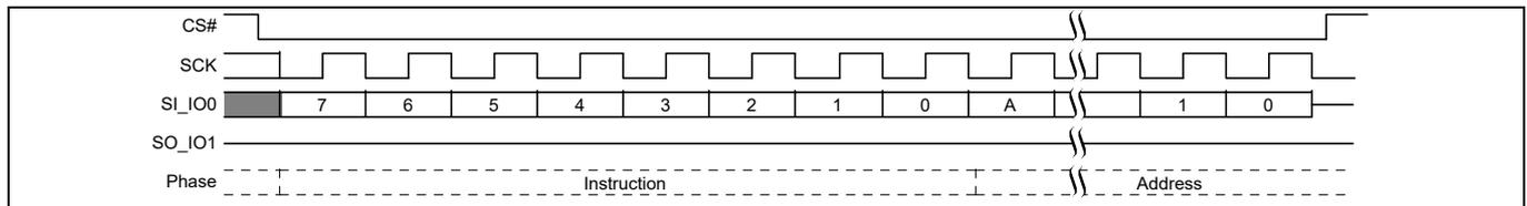
Figure 105 SPRP command sequence<sup>[59, 60]</sup>
