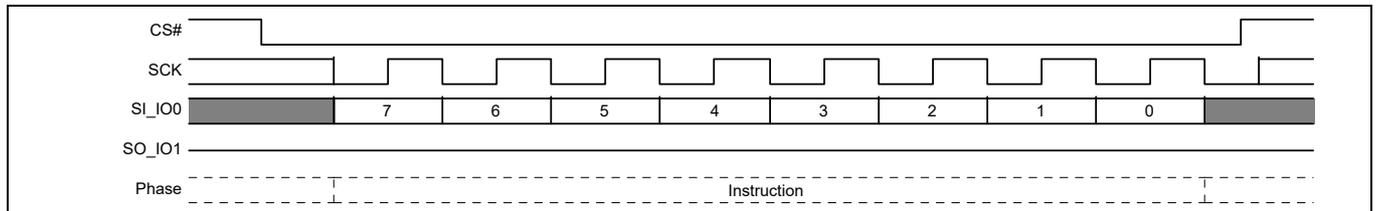
**Figure 47 Clear Status Register (CLSR) command sequence**
