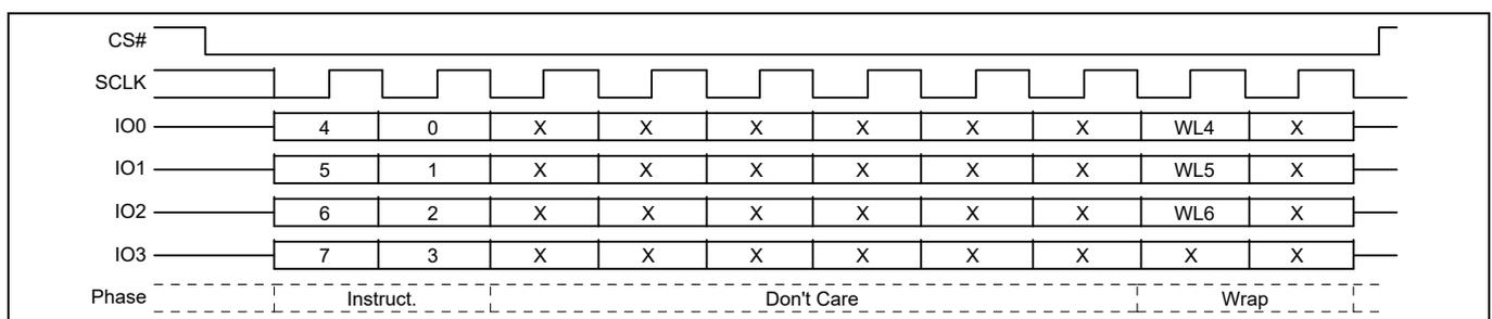
**Figure 62 Set Burst Length command sequence QPI mode**
