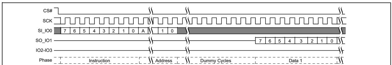
**Figure 66** Fast Read (FAST\_READ) command sequence<sup>[33]</sup>
