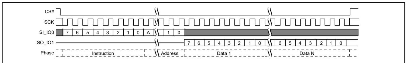
**Figure 65** Read command sequence<sup>[32]</sup>
