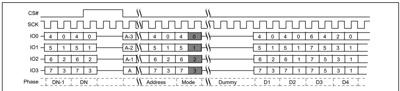
Figure 73 Continuous Quad I/O Read command sequence<sup>[38, 39]</sup>
