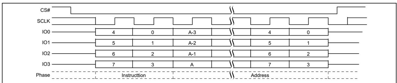
**Figure 83 Half Block Erase (HBE 52h or 4HBE 53h) QPI mode command sequence**<sup>[47, 48]</sup>
