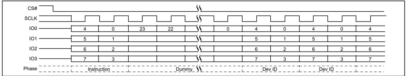
**Figure 128 Read Identification (RES) QPI mode command**
