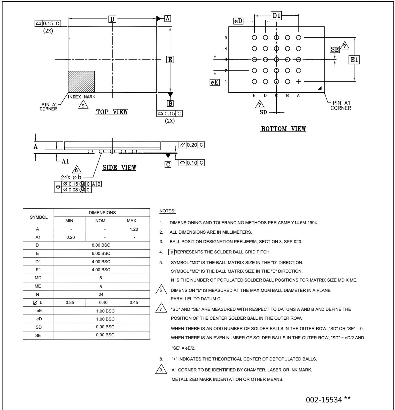
Figure 154 24-ball FBGA (8 × 6 × 1.2 mm) package outline (PG-TFBGA-24), 002-15534
