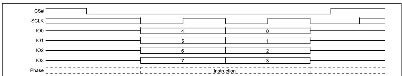
**Figure 58** Exit 4 Byte Address QPI mode
