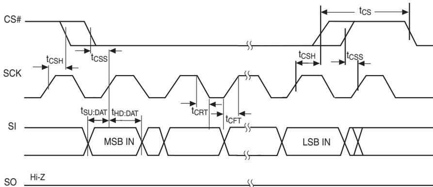
Figure 18.3 SPI Mode 0 (0,0) Output Timing
