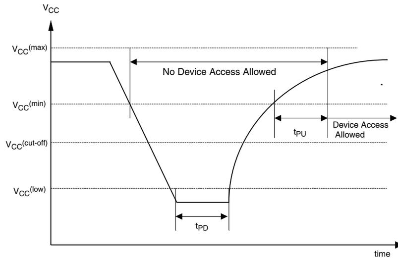
**Table 11.1 Power-Up / Power-Down Voltage and Timing**
