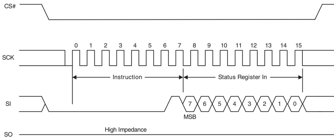
Figure 9.16 Write Registers (WRR) Instruction Sequence – 16 data bits
