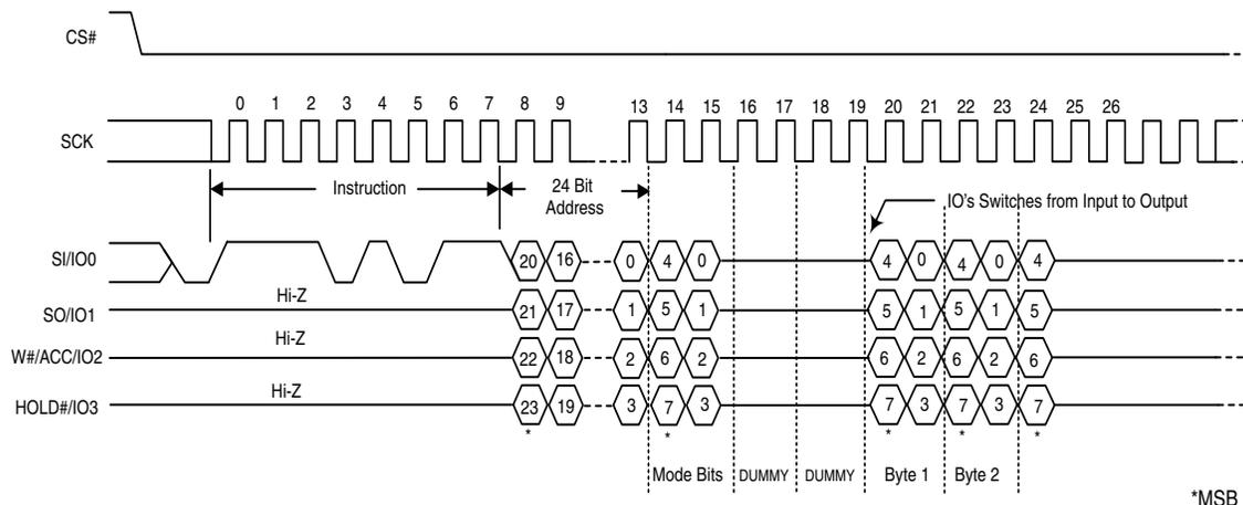
Figure 9.8 Continuous QUAD I/O High Performance Instruction Sequence
