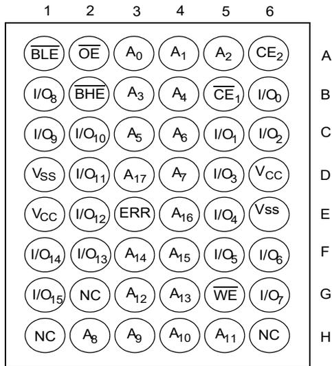
**Figure 5. 48-ball VFBGA pinout (Single Chip Enable with ERR), CY62147GE** [6, 7]
