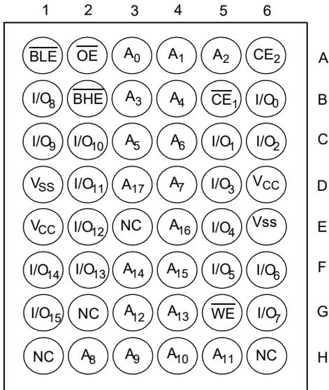
Figure 2. 48-ball VFBGA pinout (Single Chip Enable without ERR), CY62147G [5]
