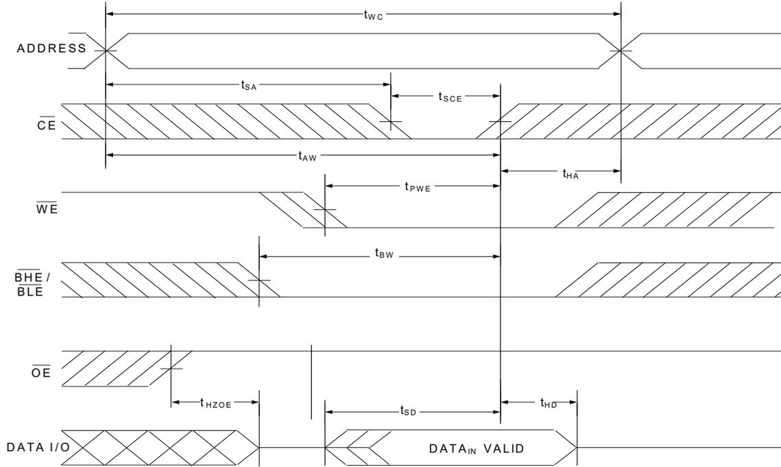
Figure 15. Write Cycle No. 3 ( $\overline{WE}$  Controlled,  $\overline{OE}$  LOW) [33, 34, 35, 36]
