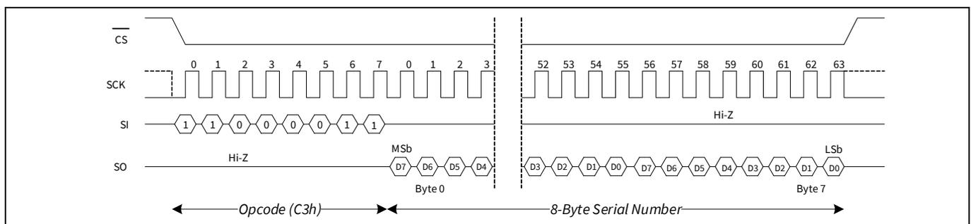
**Figure 18 Read serial number operation**
