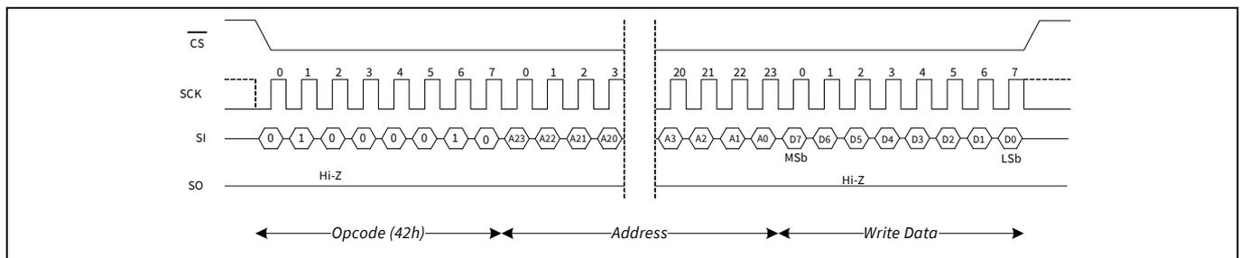
**Figure 13** Special sector write (WREN not shown) operation
