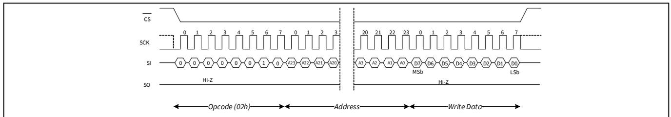
**Figure 10** Memory write (WREN not shown) operation
