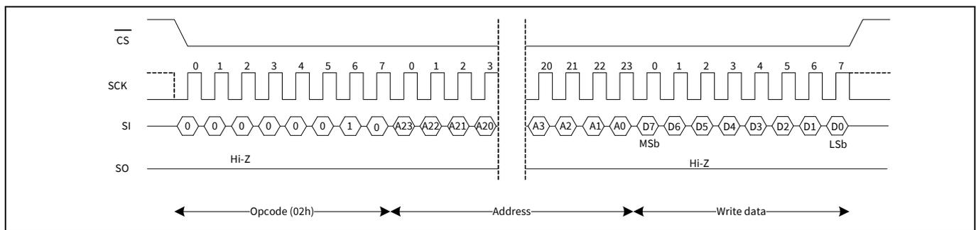
**Figure 11** Memory write (WREN not shown) operation
