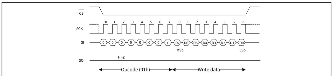
**Figure 10 WRSR bus configuration (WREN not shown)**
