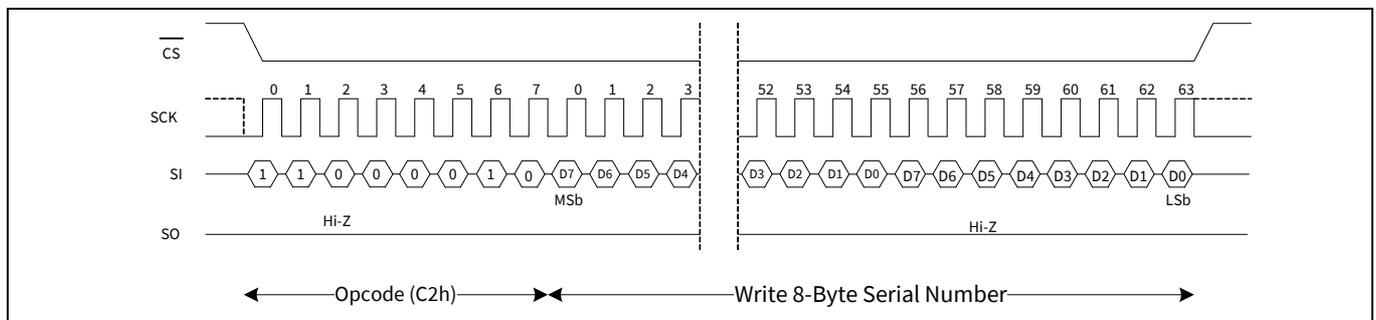
**Figure 18 Write serial number (WREN not shown) operation**
