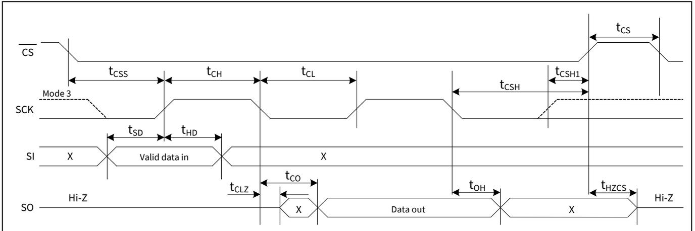
**Figure 23 Synchronous data timing (Mode 0 and Mode 3)**
