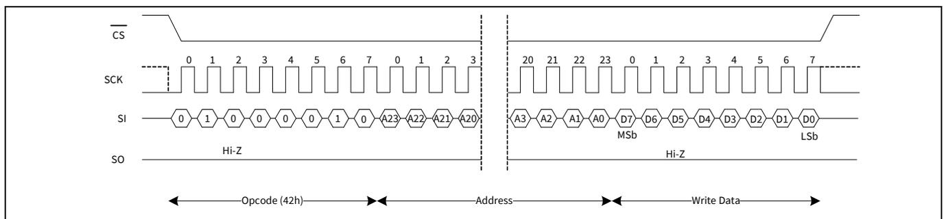
**Figure 14** Special sector write (WREN not shown) operation
