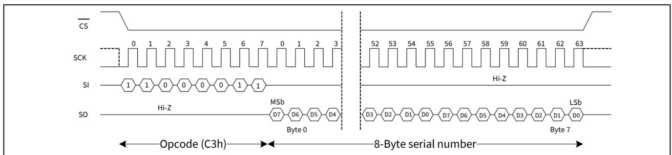
**Figure 19 Read serial number operation**
