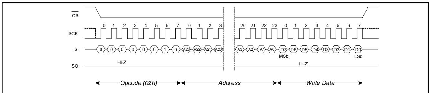
**Figure 10** Memory Write (WREN not shown) Operation
