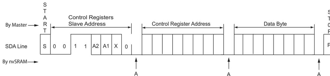
Figure 23. Multi-Byte Write into Control Registers
