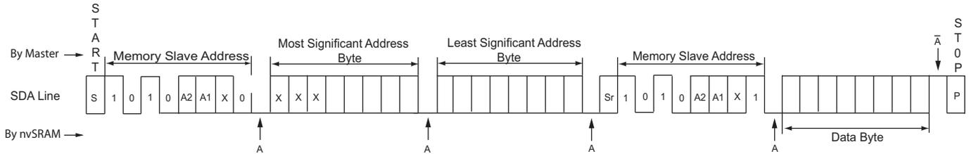
**Figure 19. Random Address Multi-Byte Read (except Hs-mode)**
