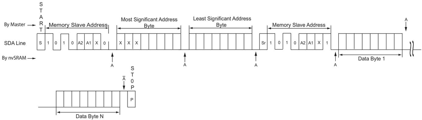
**Figure 20. Random Address Single-Byte Read (Hs-mode)**
