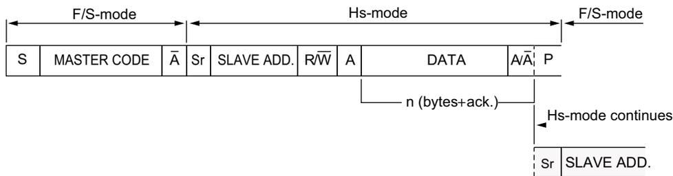
Single and multiple-byte reads and writes are supported. After the device enters into Hs-mode, data transfer continues in Hs-mode until stop condition is sent by master device. The slave switches back to F/S-mode after a STOP condition (P). To
