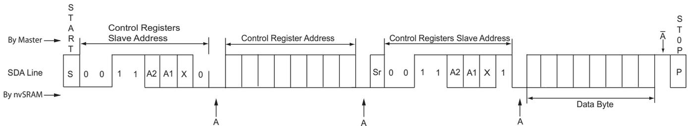
Figure 27. Random Control Registers Multi-Byte Read
