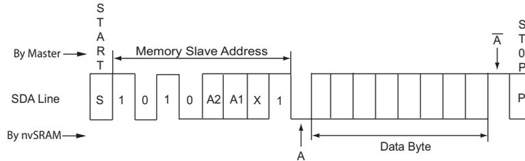
**Figure 15. Current Location Multi-Byte nvSRAM Read (except Hs-mode)**
