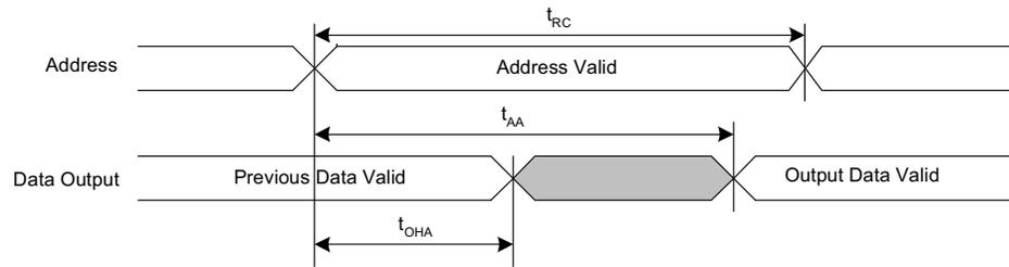
**Figure 12. SRAM Read Cycle 2:  $\overline{CE}$  and  $\overline{OE}$  Controlled**<sup>[34, 36, 37]</sup>
