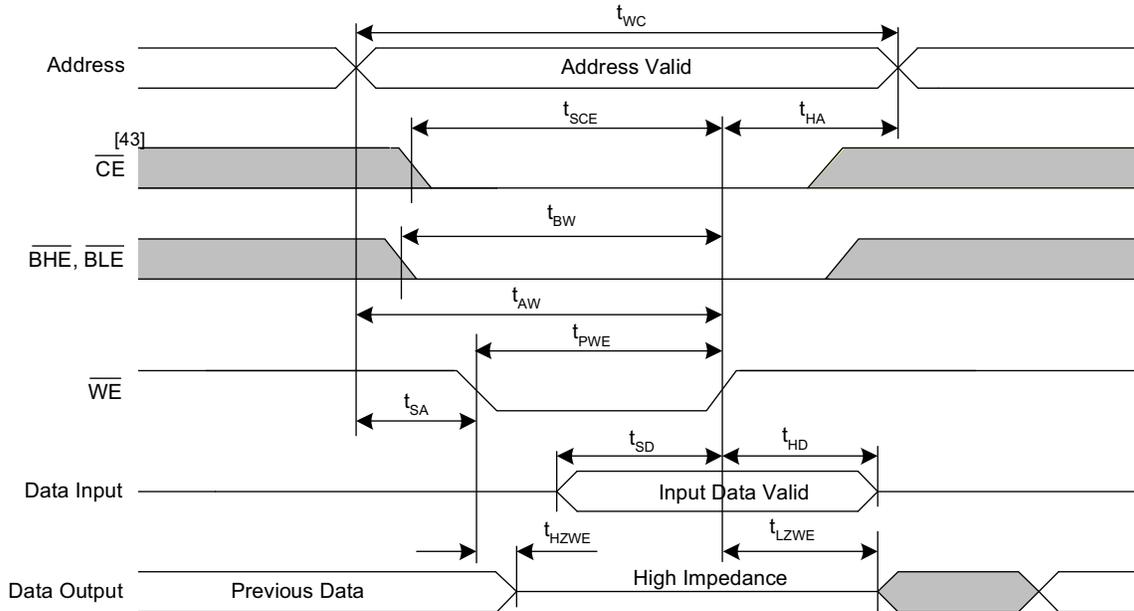
Figure 14. RAM Write Cycle 2:  $\overline{CE}$  Controlled<sup>[39, 40, 41, 42]</sup>
