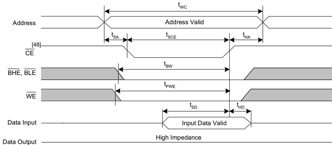
Figure 16. SRAM Write Cycle 3:  $\overline{BHE}$ ,  $\overline{BLE}$  Controlled<sup>[44, 45, 46, 47, 49]</sup>
