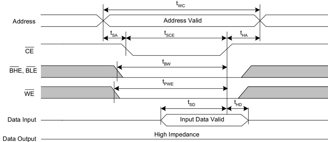
**Figure 10. SRAM Write Cycle #3 ( $\overline{\text{BHE}}$  and  $\overline{\text{BLE}}$  Controlled)** [36, 37, 38, 39]
