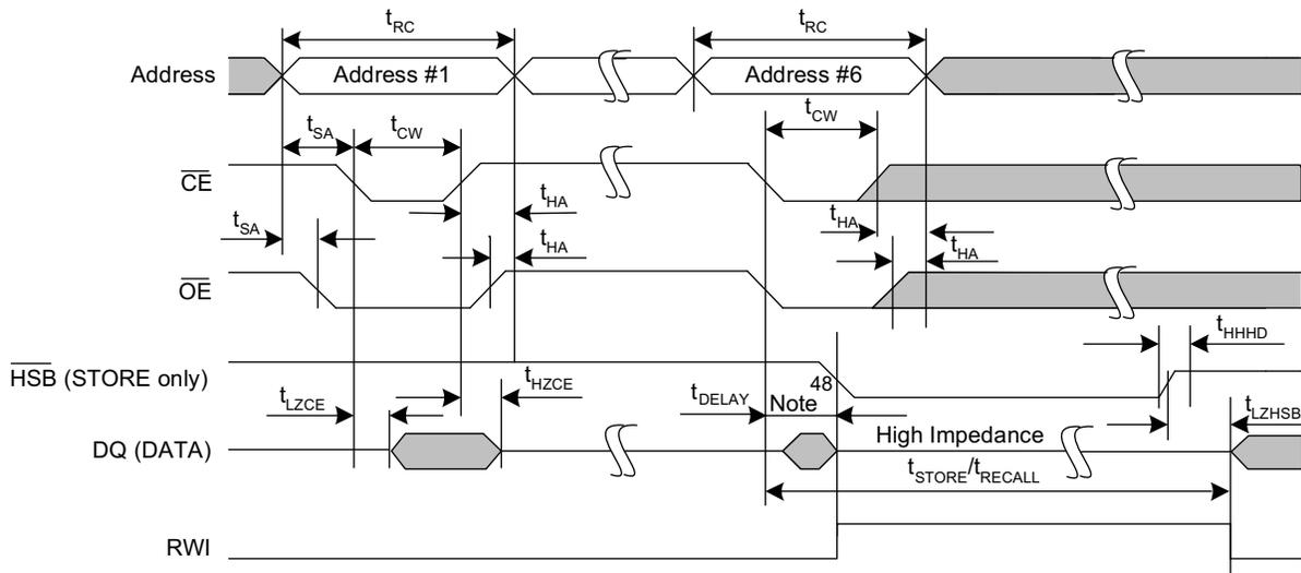
Figure 13. AutoStore Enable/Disable Cycle<sup>[47]</sup>
