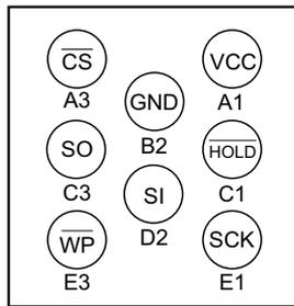
Figure 2. 8-ball WLCSP (3 x 2 x 3) — Bottom View
