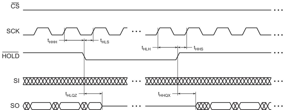
Figure 44. HOLD Timing – Serial Output
