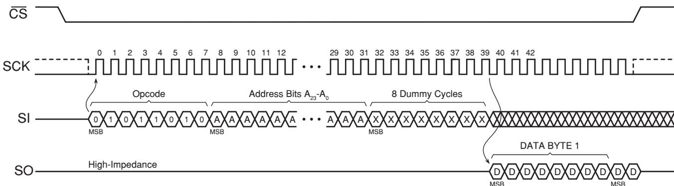
Figure 17. Read Serial Flash Discoverable Parameter Command Timing
