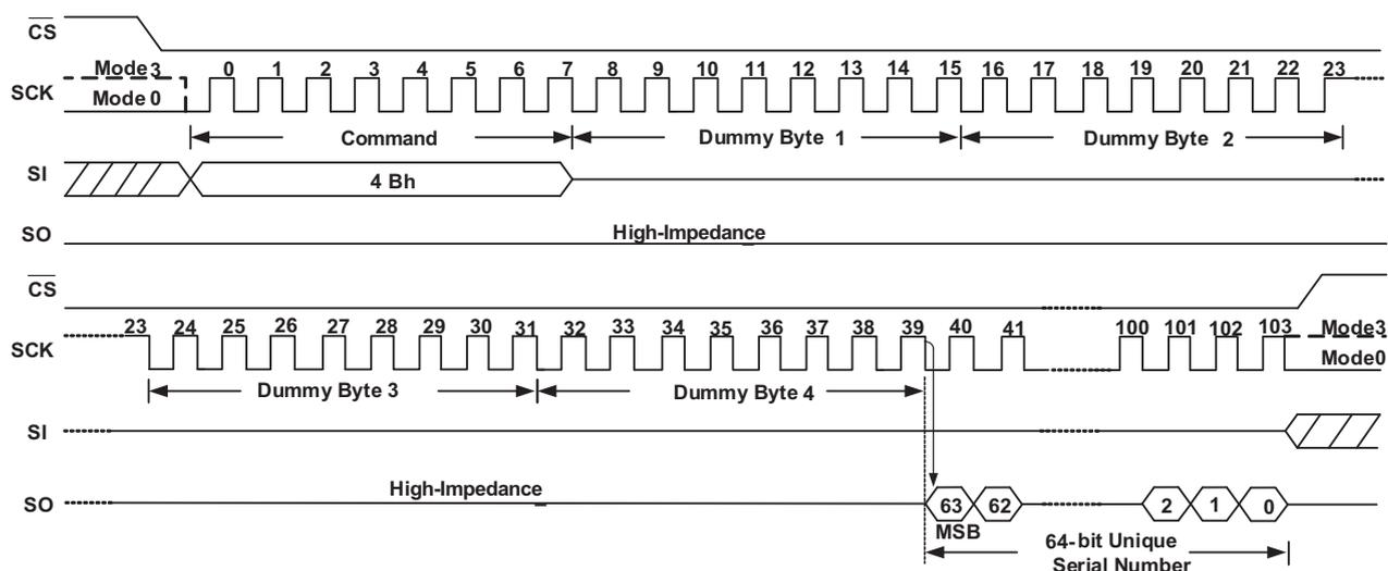
Figure 24. Read Unique ID Timing (SPI Mode)
