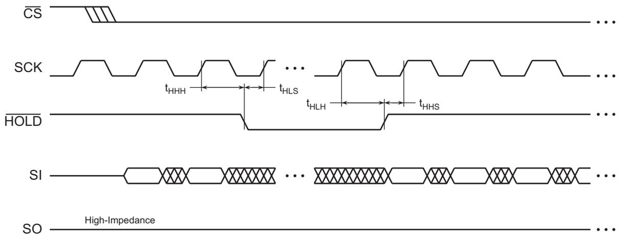
Figure 43. HOLD Timing – Serial Input
