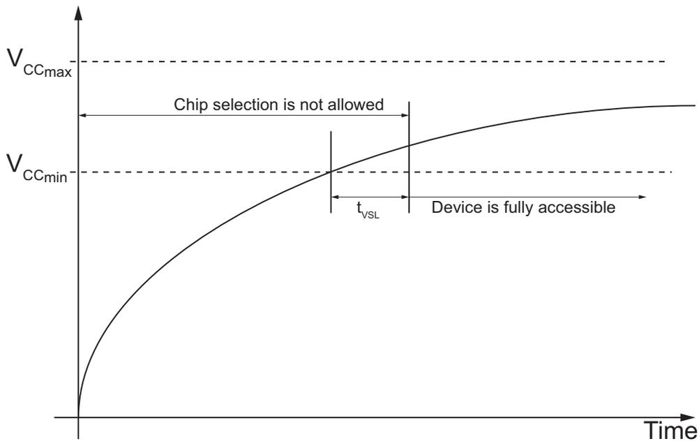
Figure 39. Power-Up Timing and Voltage
