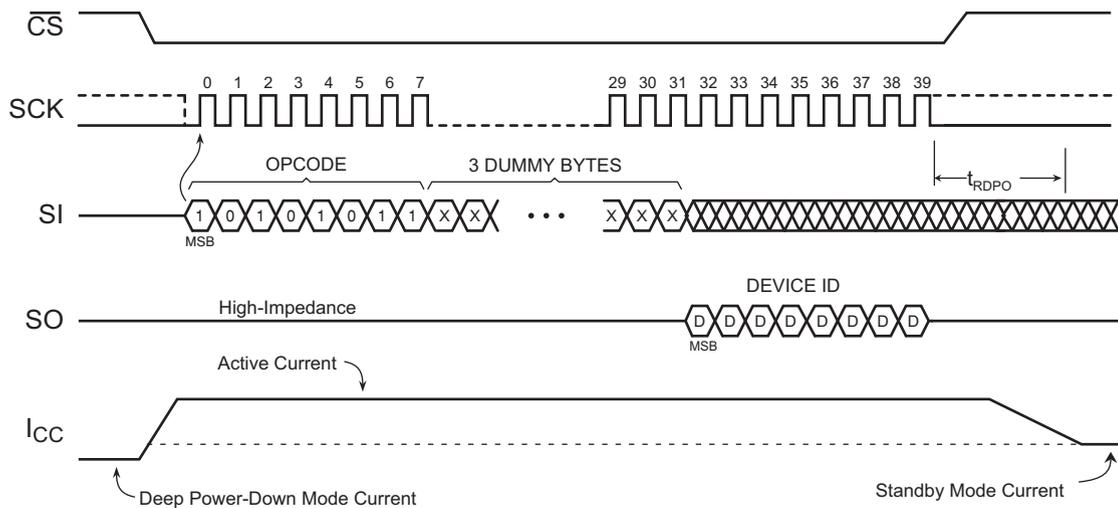
Figure 38. Resume from Deep Power-Down and Read Device ID Timing
