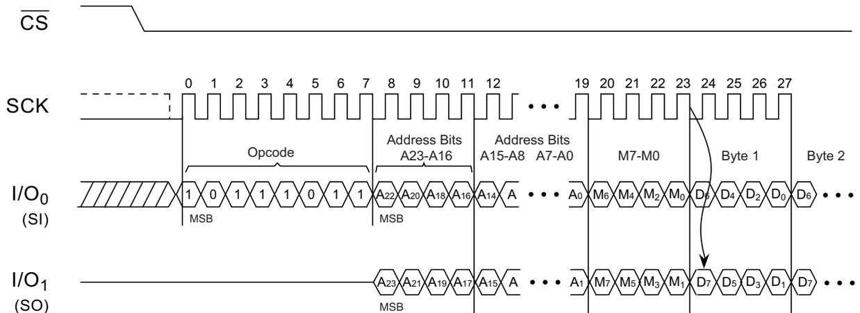
Figure 9. Dual I/O Read Array (Initial command or previous M<sub>5</sub>,M<sub>4</sub> ≠ 1,0)
