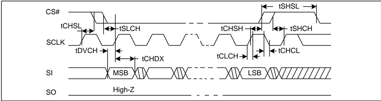
**Figure21. Output Timing**
