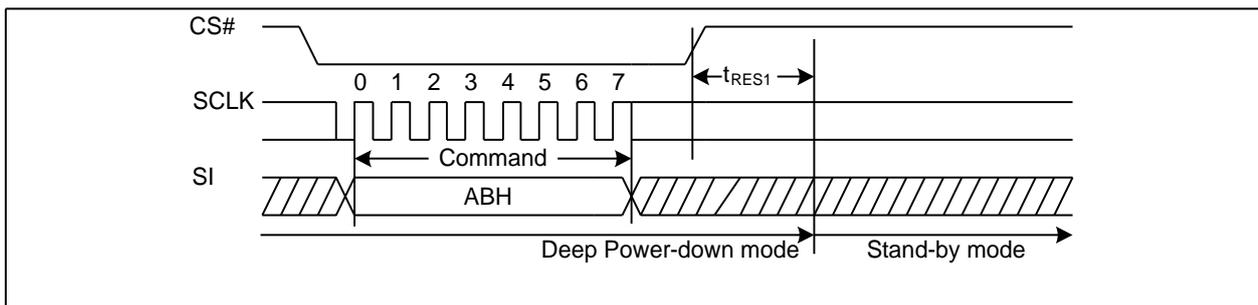
**Figure15. Release Power-Down and Read Device ID Sequence Diagram**
