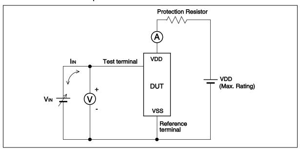
Note: The voltage VIN is increased gradually and the current  $I_{IN}$  of 300 mA at maximum shall flow. Confirm the latch up does not occur under  $I_{IN}$  =  $\pm$  300 mA.
