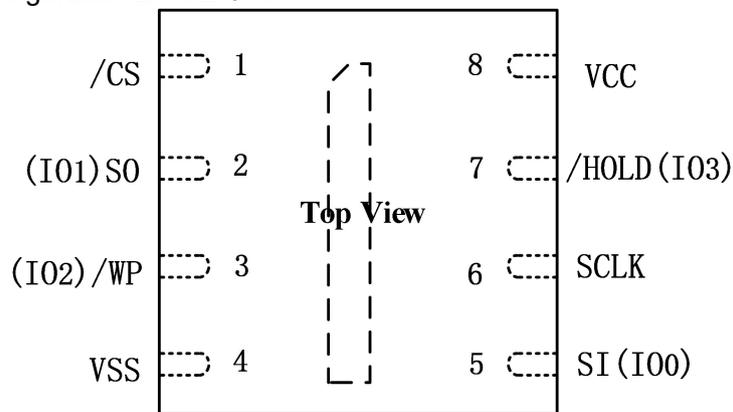
**Figure 3.b.** Pin Configuration DFN 1.5\*1.5mm
