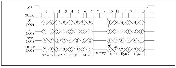
Quad I/O Word Fast Read with "8/16/32/64-Byte Wrap Around" in standard SPI mode
