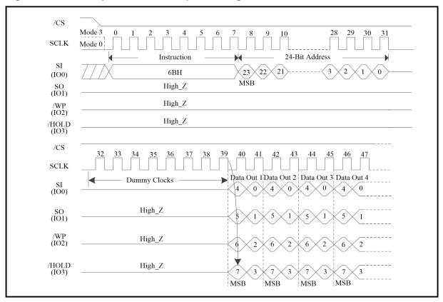
Figure 15. Quad Output Fast Read Sequence Diagram
