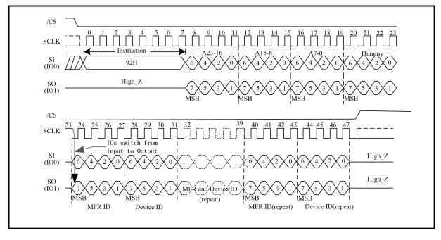
Figure 24. Dual I/O Read Manufacture ID/ Device ID Sequence Diagram
