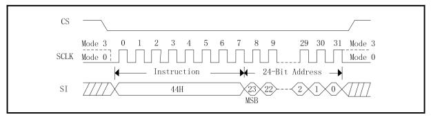
Figure 32. Erase Security Registers instruction Sequence Diagram
