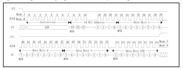
Figure 33. Program Security Registers instruction Sequence Diagram
