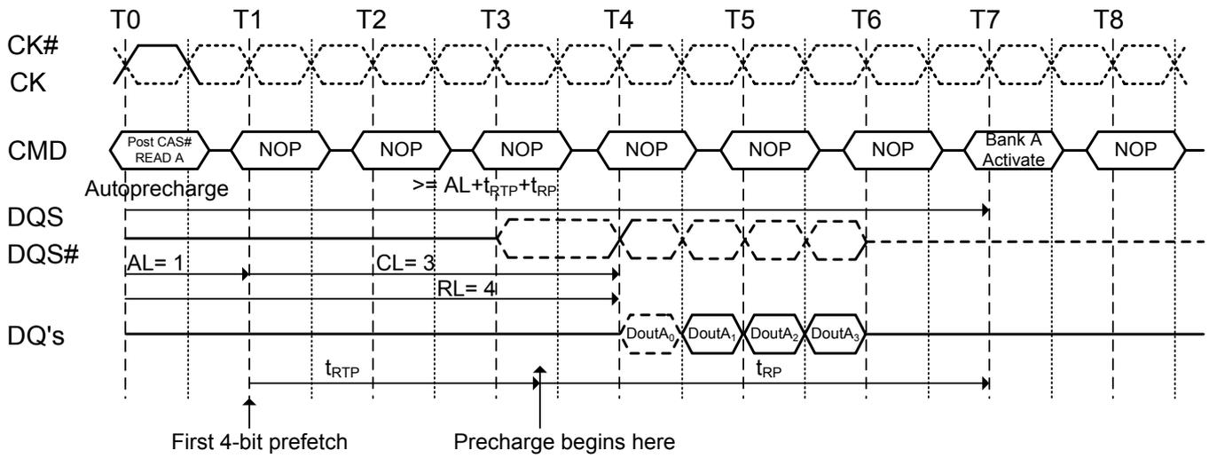
**Figure 44. Burst read operation with auto precharge followed by activation to the same bank ( $t_{RC}$  Limit): RL=5(AL=2, CL=3, internal  $t_{RCD}=3$ , BL=4,  $t_{RTP} \leq 2$  clocks)**
