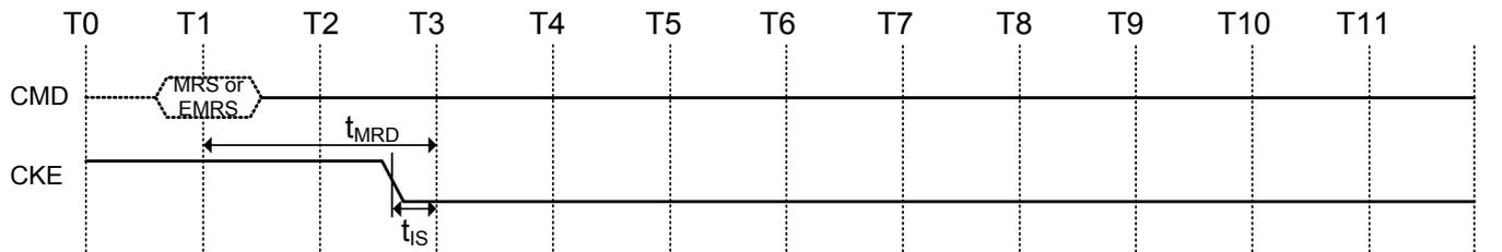
**Figure 61. Asynchronous CKE LOW event**
