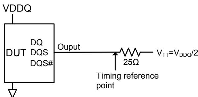
The output timing reference voltage level for single ended signals is the crosspoint with VTT. The output timing reference voltage level for differential signals is the cross point of the true (e.g. DQS) and the complement (e.g. DQS#) signal.
