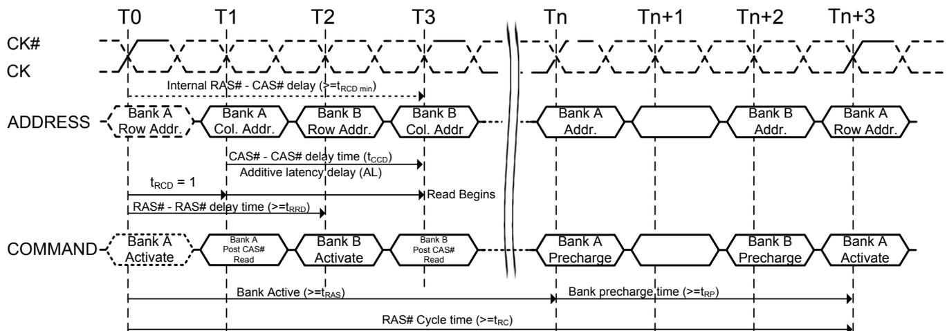
**Figure 20. Posted CAS# operation: AL=2, Read followed by a write to the same bank**
