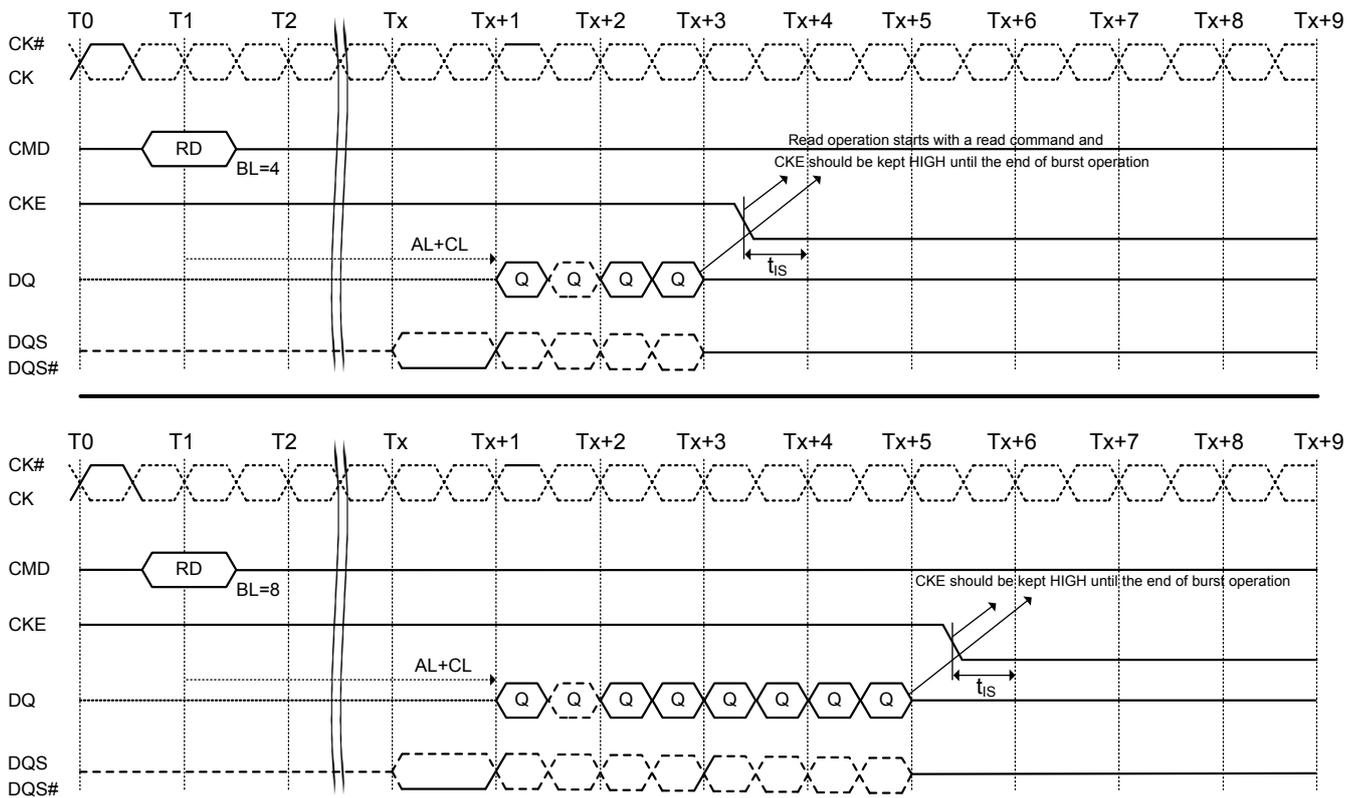
**Figure 54. Read with autoprecharge to power-down entry**
