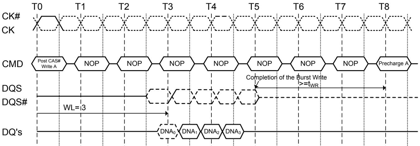
**Figure 41. Burst write followed by precharge:  $WL = (RL-1) = 4$**
