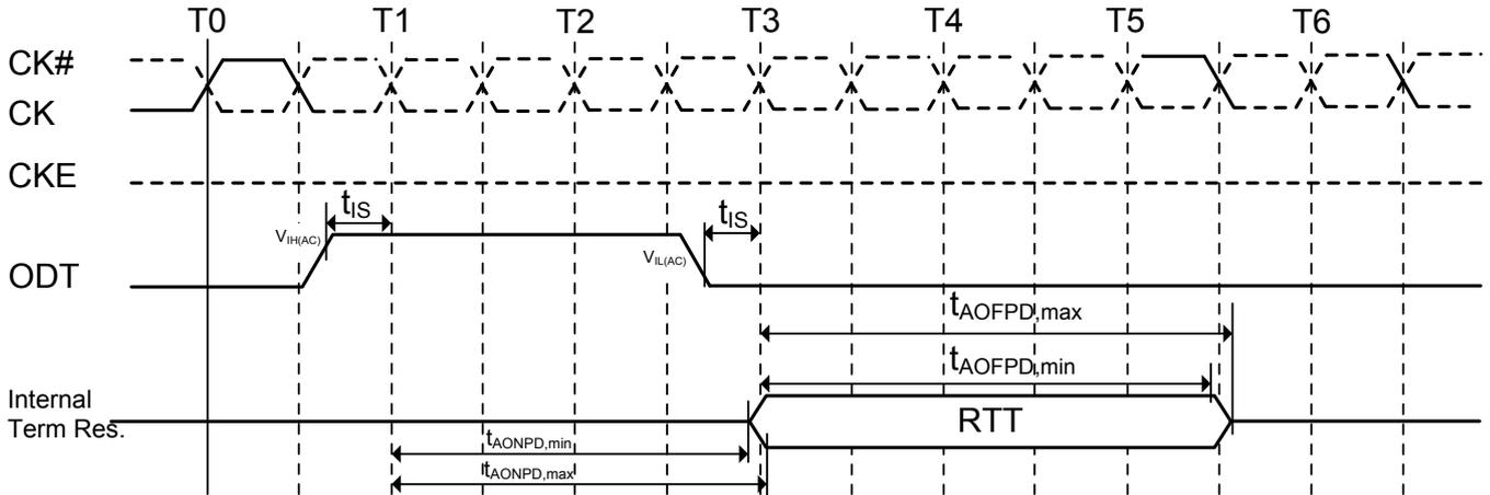
**Figure 17. ODT timing mode switch at entering power-down mode**
