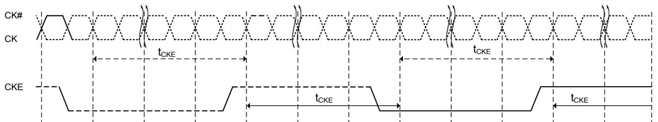
NOTE: DRAM guarantees all AC and DC timing & voltage specifications and proper DLL operation with intensive CKE operation
