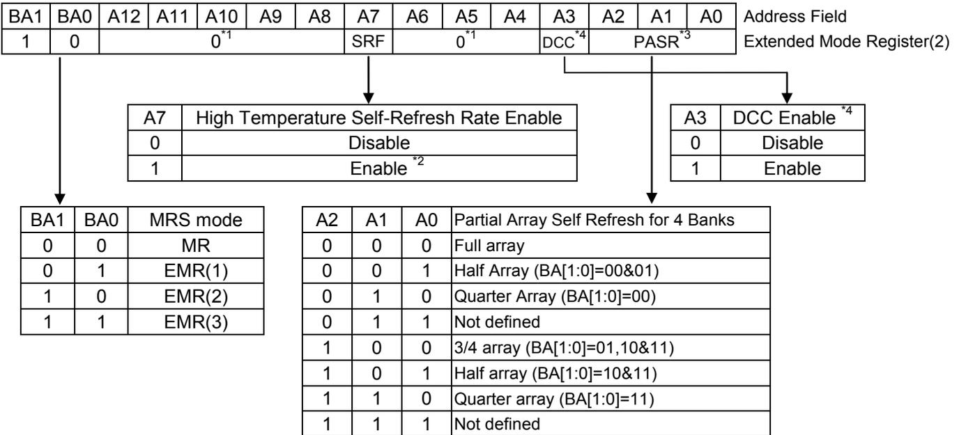
**NOTE 1:** The rest bits in EMRS(2) are reserved for future use and all bits in EMRS(2) except A0-A2, A7, BA0 and BA1 must be programmed to 0 when setting the extended mode register(2) during initialization.
