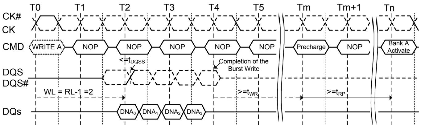
Figure 31. Burst write followed by burst read: RL=5 (AL=2, CL=3, WL=4,  $t_{WTR}$ =2, BL=4)
