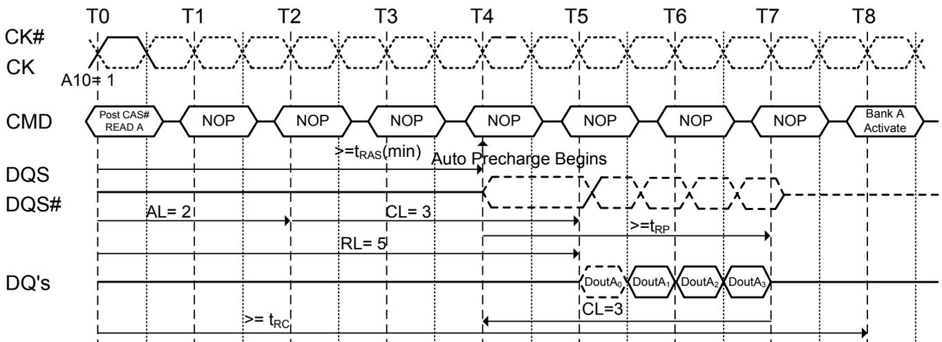
**Figure 45. Burst read operation with auto precharge followed by an activation to the same bank ( $t_{RP}$  Limit): (RL=5 (AL=2, CL=3, internal  $t_{RCD}$ =3, BL=4,  $t_{RTP} \leq 2$  clocks)**
