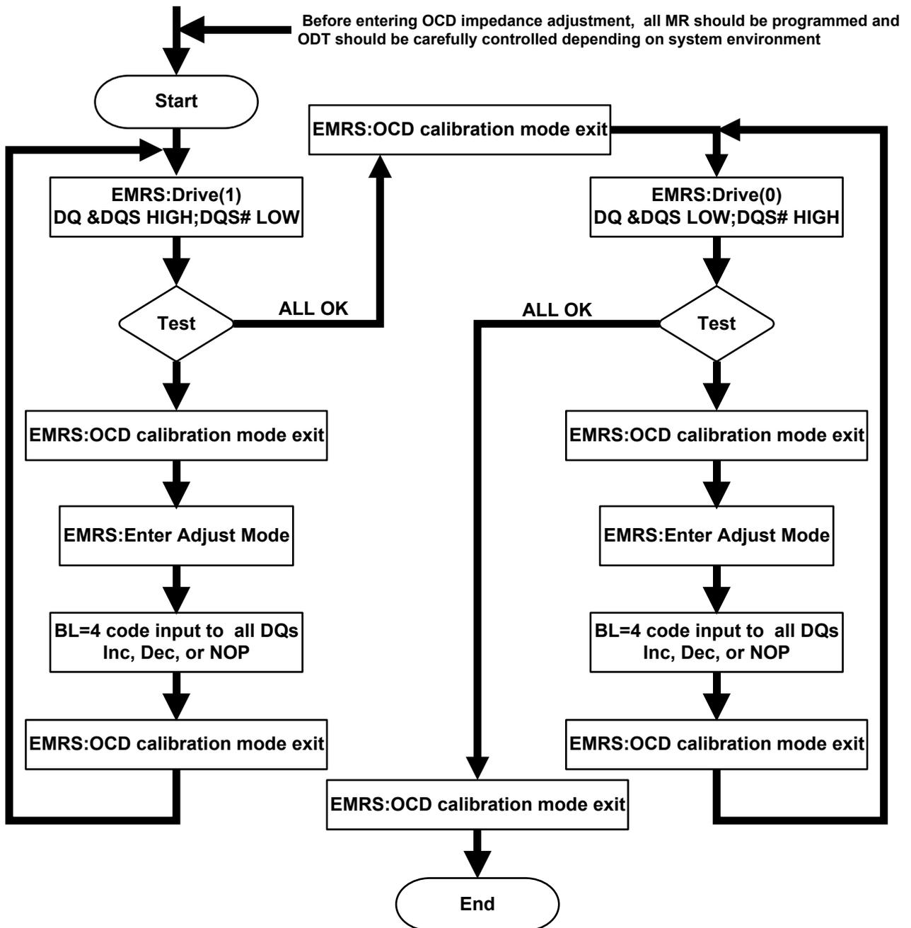
**- Extended mode register for OCD impedance adjustment**
