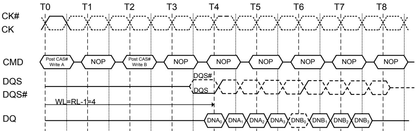
NOTE : The seamless burst write operation is supported by enabling a write command every other clock for BL= 4 operation, every four clocks for BL = 8 operation. This operation is allowed regardless of same or different banks as long as the banks are activated.
