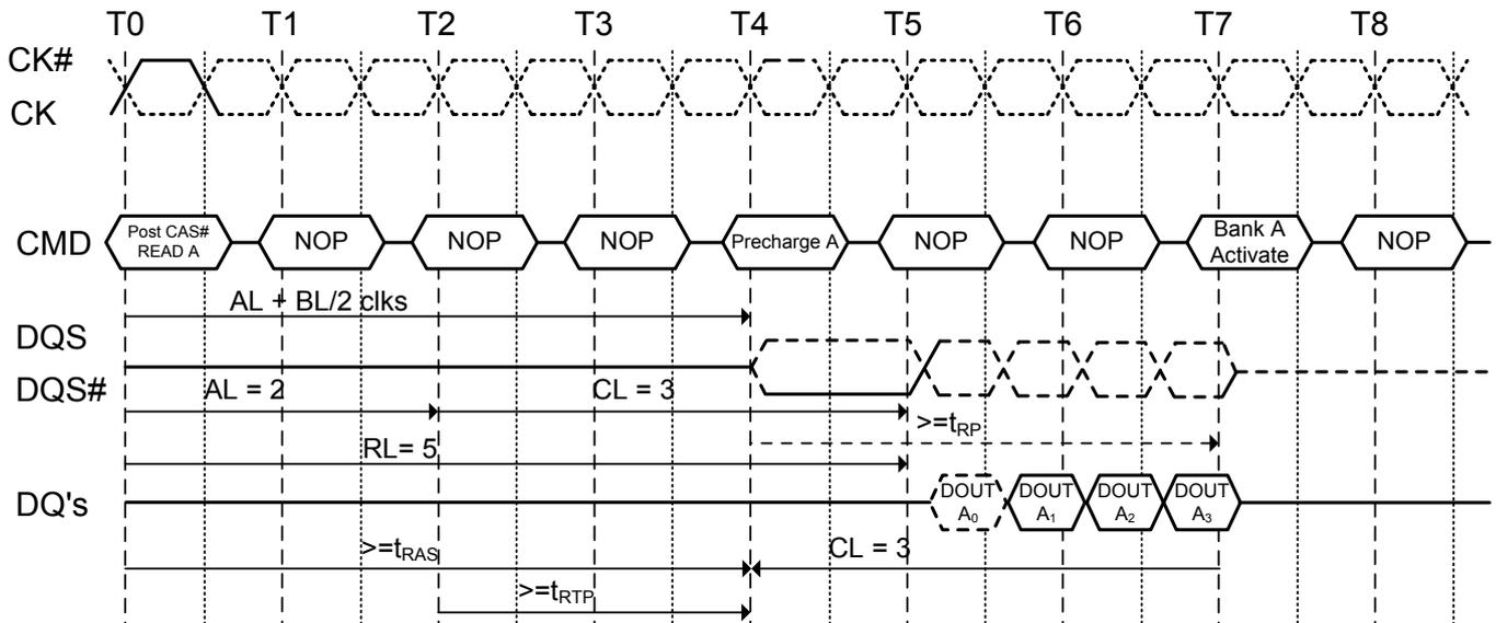
**Figure 38. Burst read operation followed by precharge:**
