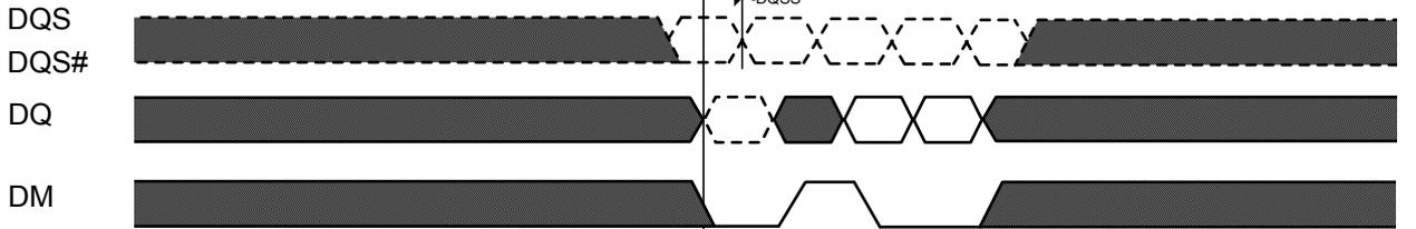
**Figure 35. Burst read operation followed by precharge:**
