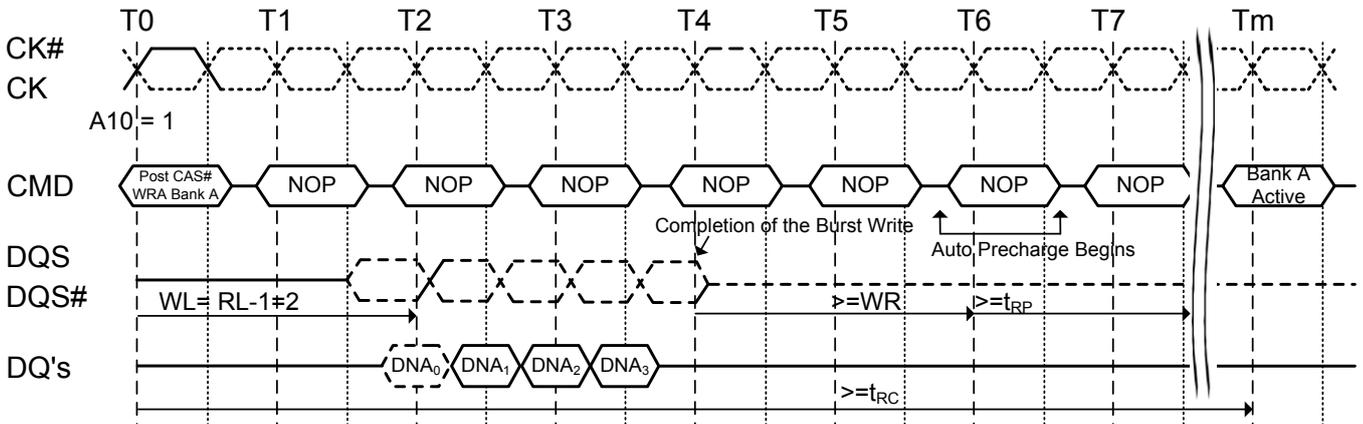
Figure 47. Burst write with auto-precharge ( $WR+t_{RP}$ ):  $WL=4$ ,  $WR=2$ ,  $BL=4$ ,  $t_{RP}=3$
