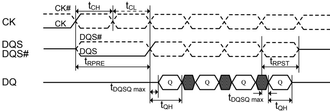
Figure 23. Burst read operation: RL=5 (AL=2, CL=3, BL=4)
