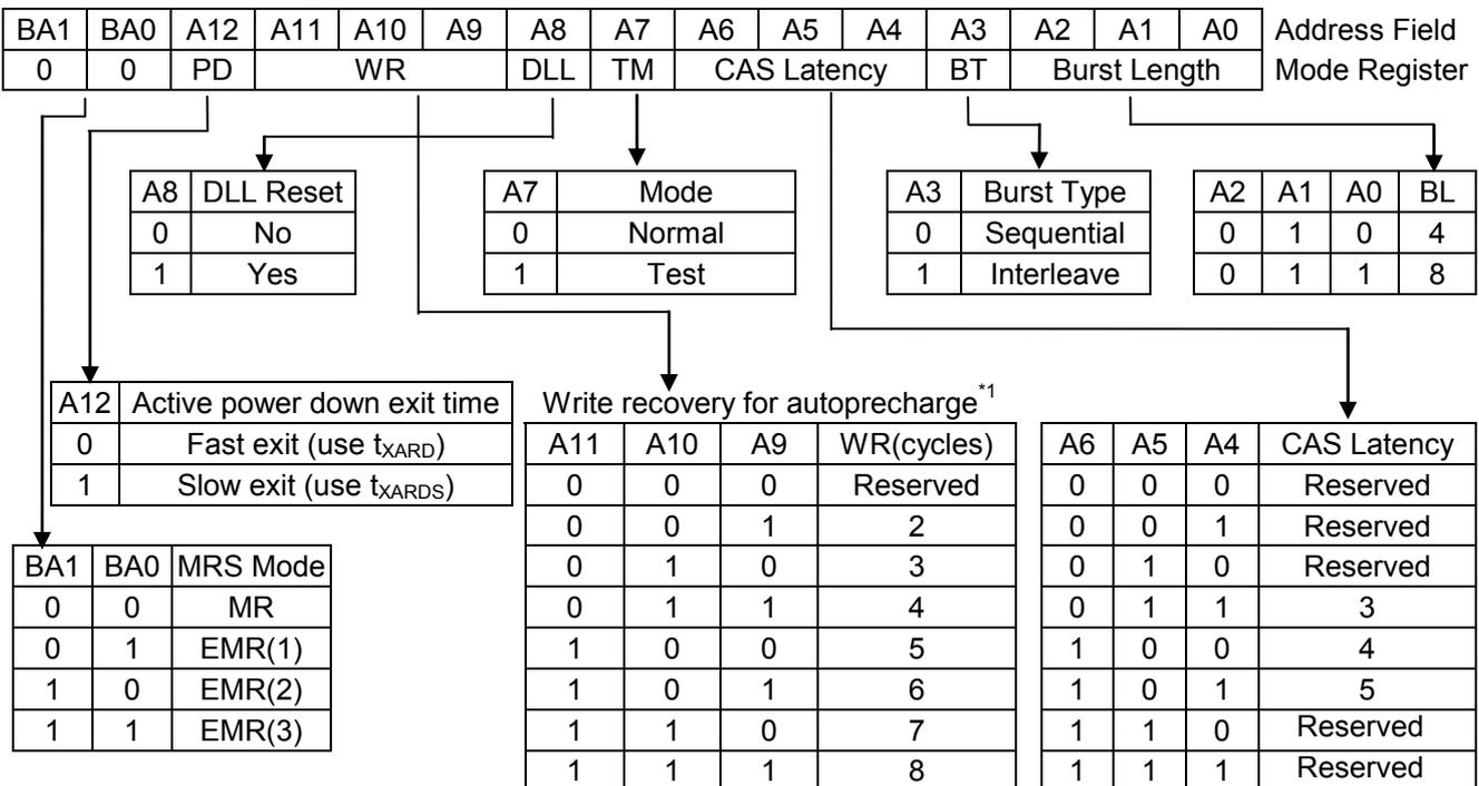
**NOTE 1:** For DDR2-800, WR min is determined by  $t_{CK}(\text{avg})$  max and WR max is determined by  $t_{CK}(\text{avg})$  min.  $WR$  [cycles] =  $RU \{t_{WR}[\text{ns}]/t_{CK}(\text{avg})[\text{ns}]\}$ , where RU stands for round up. The mode register must be programmed to this value. This is also used with  $t_{RP}$  to determine  $t_{DAL}$ .
