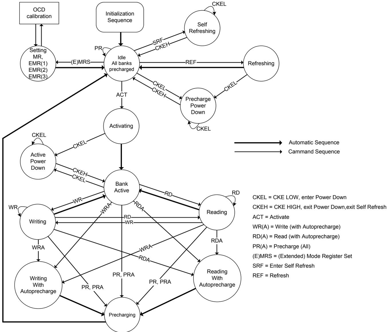
Note: Use caution with this diagram. It is intended to provide a floorplan of the possible state transitions and the commands to control them, not all details. In particular situations involving more than one bank, enabling/disabling on-die termination, Power Down entry/exit, timing restrictions during state transitions, among other things, are not captured in full detail.
