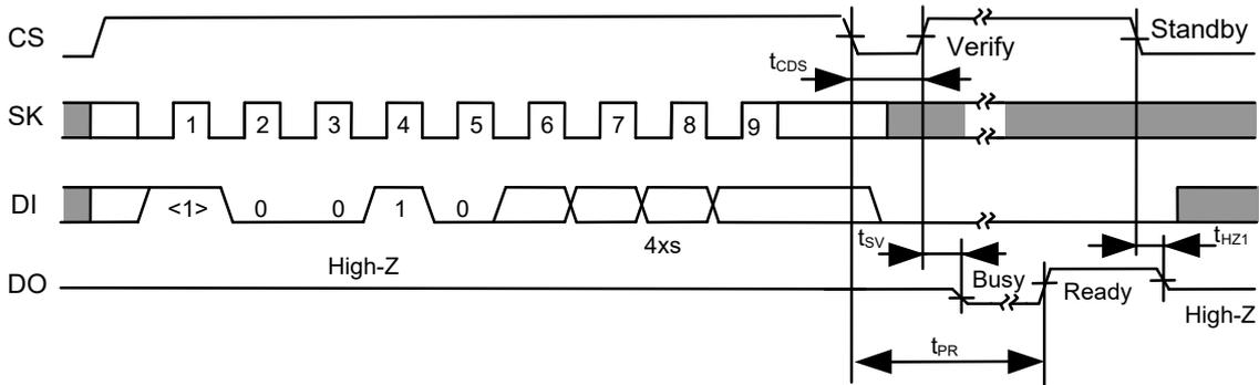
**Figure 14 Chip Erase Timing (S-93A46B)**
