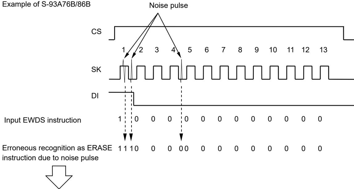
In products that do not incorporate a clock pulse monitoring circuit, "FFFFh" is mistakenly written to address 00h. However the S-93A76B/86B detects the overcount and cancels the instruction without performing a write operation.
