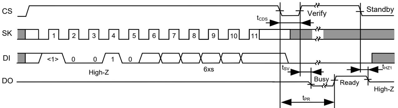
**Figure 15 Chip Erase Timing (S-93A56B/66B)**
