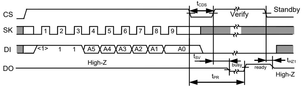
**Figure 8 Data Erase Timing (S-93A46B)**
