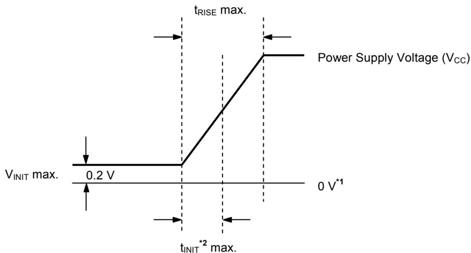
\*1. 0 V means there is no difference in potential between the VCC pin and the GND pin of the S-24C32C/64C.
