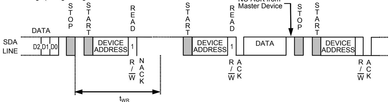
**Remark** Users are able to input word address and data after ACK output in acknowledge polling during write. Users are able to read data after ACK output in acknowledge polling during read. However, after that users input the write instruction, a start condition may not be input during data output. Input a stop condition and the next instruction after data output and ACK output.
