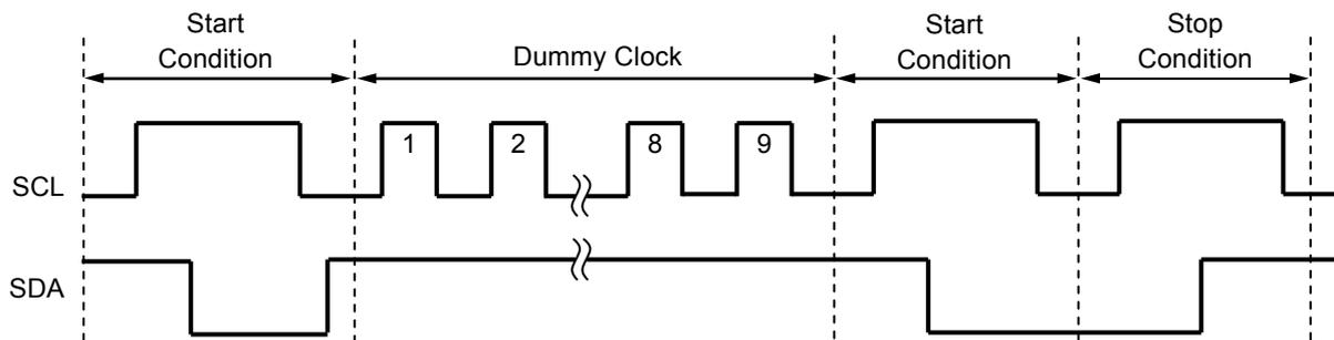
**Figure 26 Resetting S-24C32C/64C**
