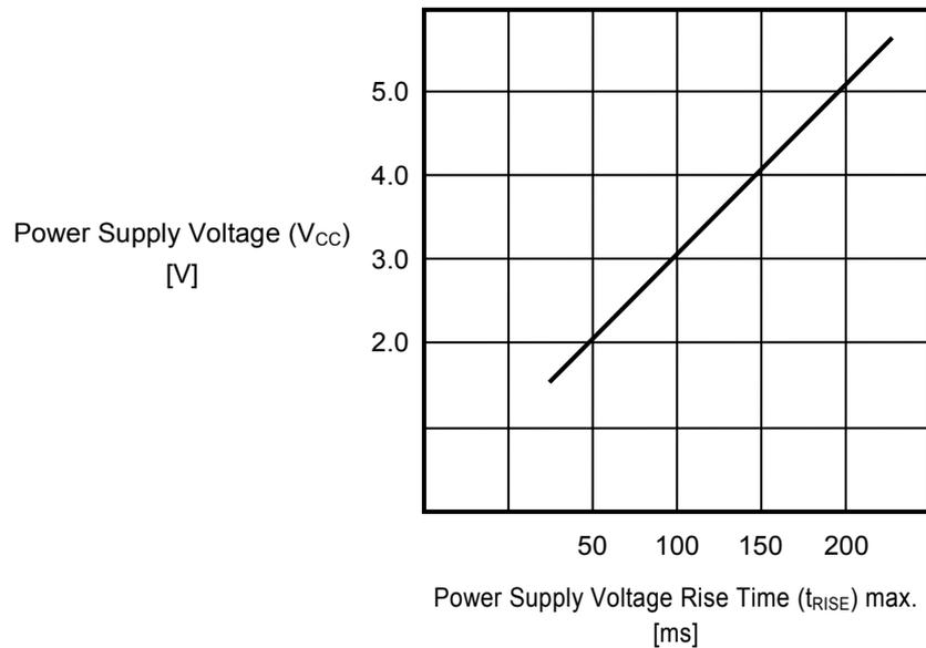
For example: If the power supply voltage = 5.0 V, raise the voltage to 5.0 V within 200 ms.
