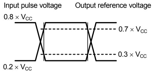
Figure 6 I/O Waveform during AC Measurement
