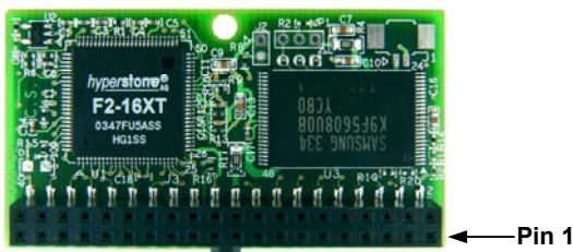
Figure 4: iDiskOnChip Horizontal Version 40 pin, Right-Oriented
