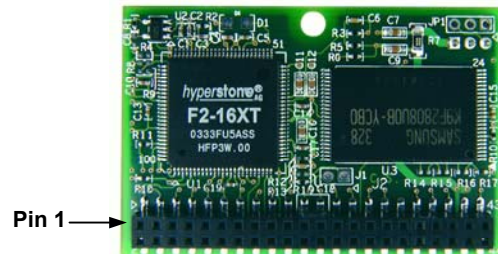
Figure 5: iDiskOnChip Horizontal Version 44 pin, Left-Oriented
