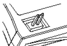
Figure 8: Master Setting for Vertical iDiskOnChip 44-Pin Connector
