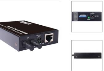
Extends a 10/100 Mbps Ethernet network connection over ST duplex multimode fiber optic cable up to 2 kilometers.
