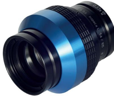
The four variants of the inspec.x L 5.6/105 are optimized for magnifications of 0.33x, 0.5x, 0.76x and 1x respectively. The V-groove interface at both ends of the lens enables adjustment to the best azimuth position and use of the lens in retro position for magnifications up to 3x. All lenses feature lockable iris and are engineered for the use in harsh industrial environments.
