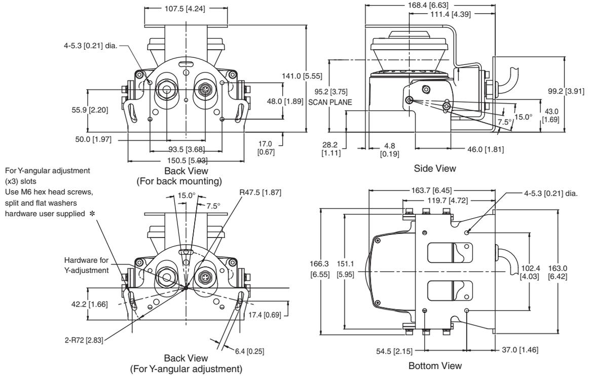
\* In order to comply with Section 4.2.16 of IEC 61496-3, when the OS32C is mounted where the scanner position could change (e.g. as the result of an impact), additional mechanical means, such as serrated or toothed lock washers, must be employed in the mounting hardware.
