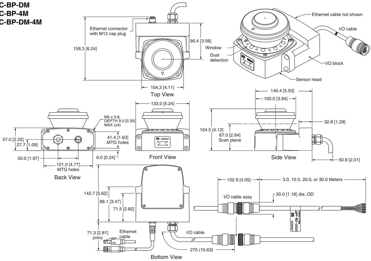
OS32C with Side Location Cable Entry/with EtherNet/IP and Side Location Cable Entry
