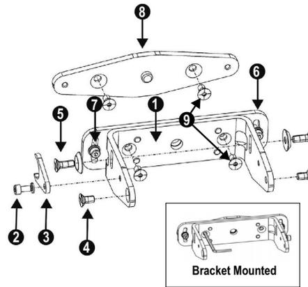
Figure 2: Pitch and roll angle adjustment bracket (SXA-MBK-1)
