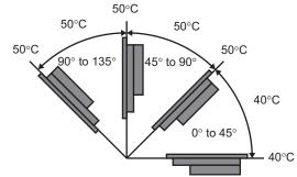
**\*2.** Use the Programmable Terminal within the following temperature and humidity ranges.
