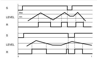
The output relay energizes when the liquid level reaches the high probe. The relay de-energizes when the liquid falls below the low probe. This control can also be used with only two probes by connecting the maximum and common terminals together. The output is energized when the level reaches the low probe. In both functions, if the container is conductive, it may be used as the common probe in some applications.
