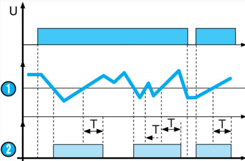
**Monitoring a level, filling function, deactivation time**
