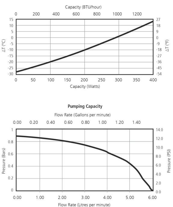
**Thermal Capacity** △T=Outlet Fluid Temperature - Ambient Temperature
