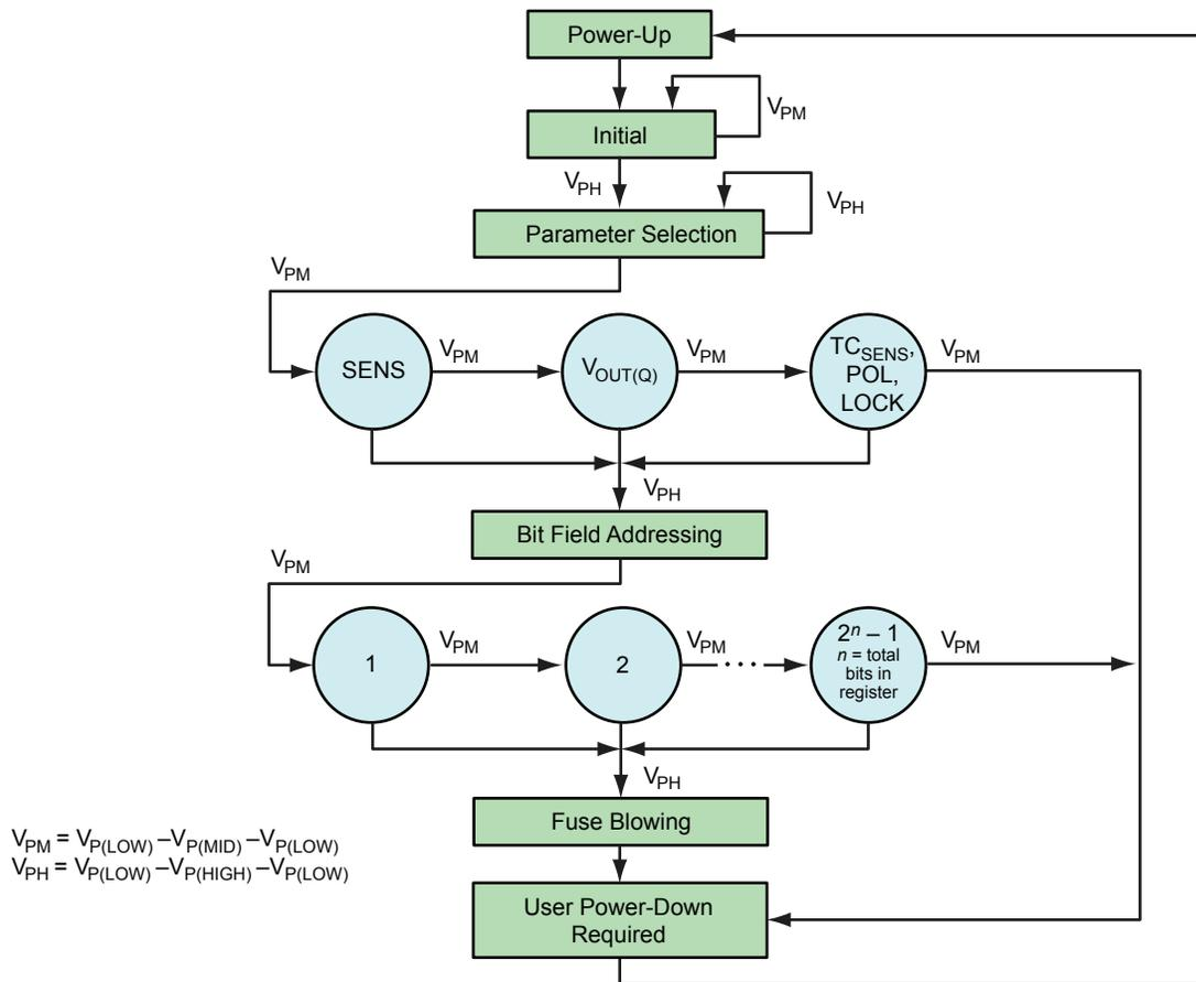
**Initial State** After system power-up, the programming logic is reset to a known state. This is referred to as the Initial state. All the bit field locations that have intact fuses are set to logic 0. While in the Initial state, any  $V_{PM}$  pulses on the VOUT pin are ignored. To enter the Parameter Selection state, apply one  $V_{PH}$  pulse on the VOUT pin.
