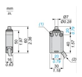
(1) 2 fixing holes Ø 4.2 mm, counterbored Ø 8 mm by 4 mm deep.(2) External diameter of cable 7.5 mm.
