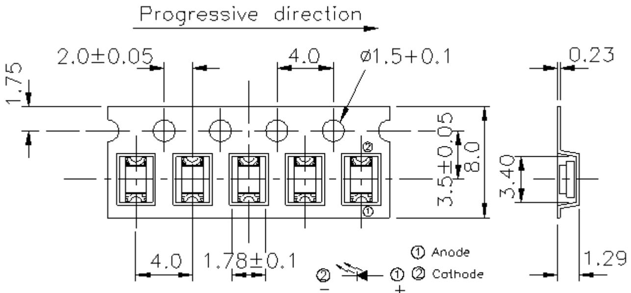
**Note:** The tolerances unless mentioned are  $\pm 0.1$ mm, Unit: mm
