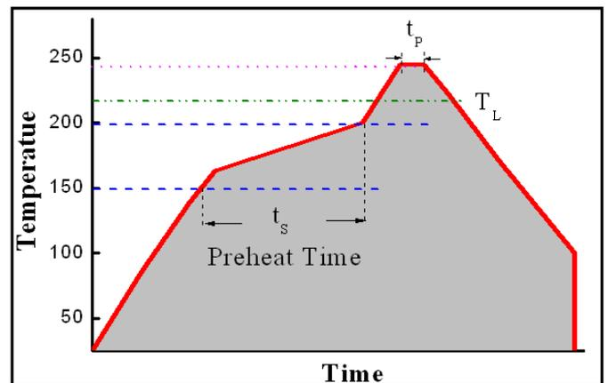
3. Reflow soldering should not be done more than twice.
