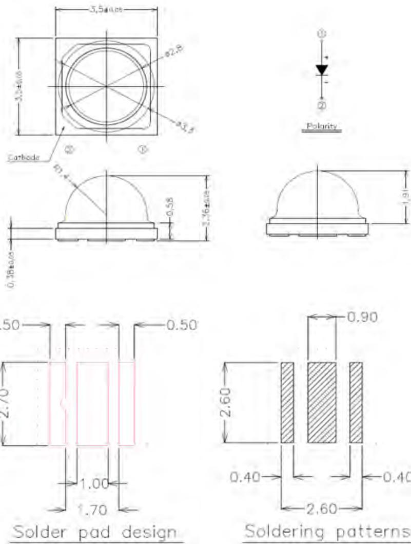
1. Dimensions are in millimeters.
