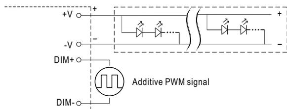
"DO NOT connect "DIM- to -V"
