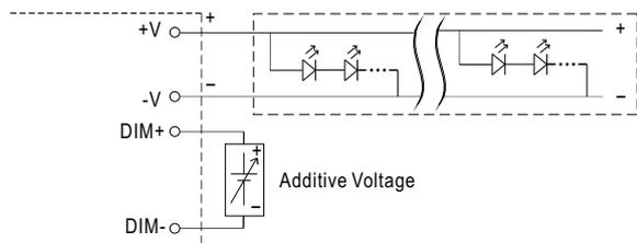
"DO NOT connect "DIM- to -V"
