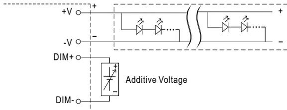
"DO NOT connect "DIM- to -V"
