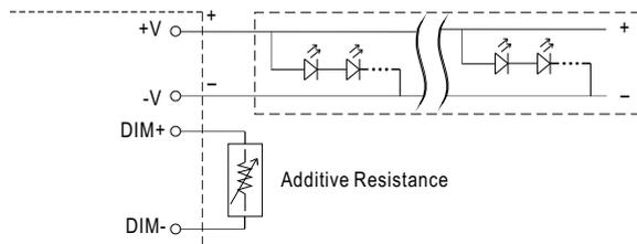
"DO NOT connect "DIM- to -V"
