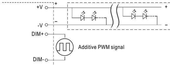
"DO NOT connect "DIM- to -V"
