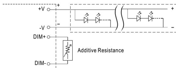
"DO NOT connect "DIM- to -V"
