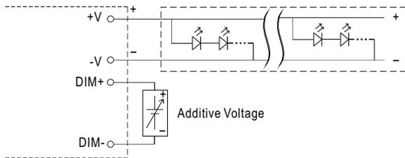
"DO NOT connect "DIM- to -V"
