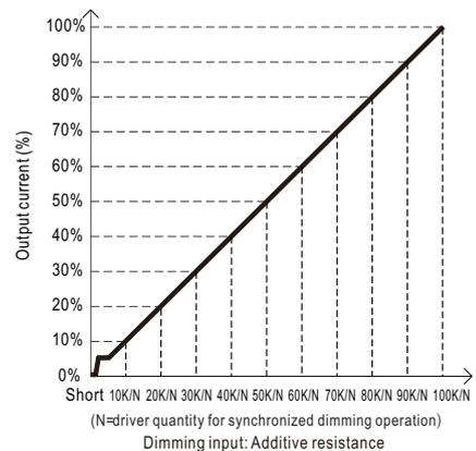
Note : 1. Min. dimming level is about 5% and the output current is not defined when 0% < I<sub>out</sub> < 5%.
