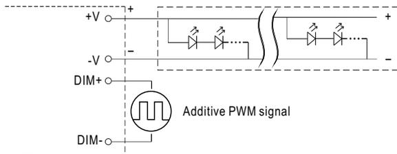
"DO NOT connect "DIM- to -V"
