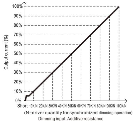
Note : 1. Min. dimming level is about 8% and the output current is not defined when 0% < I<sub>out</sub> < 8%.
