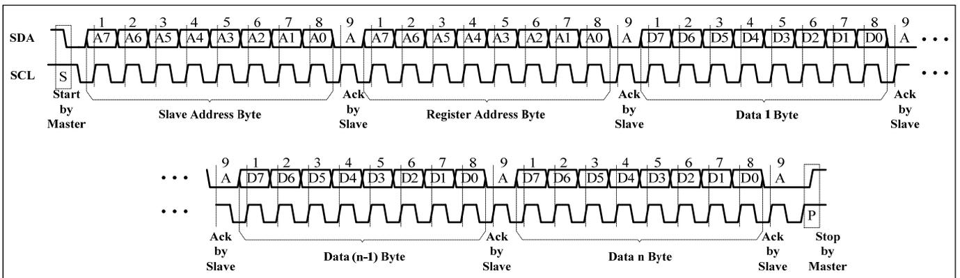
Figure 7 Writing to IS31FL3723 (Automatic Address Increment)
