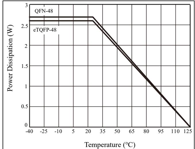
Figure 17 Dissipation Curve
