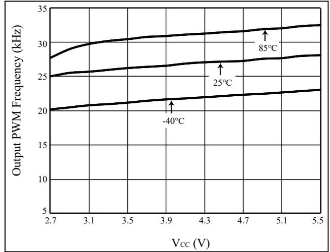
**Figure 18** V<sub>CC</sub> vs. CSx PWM Frequency
