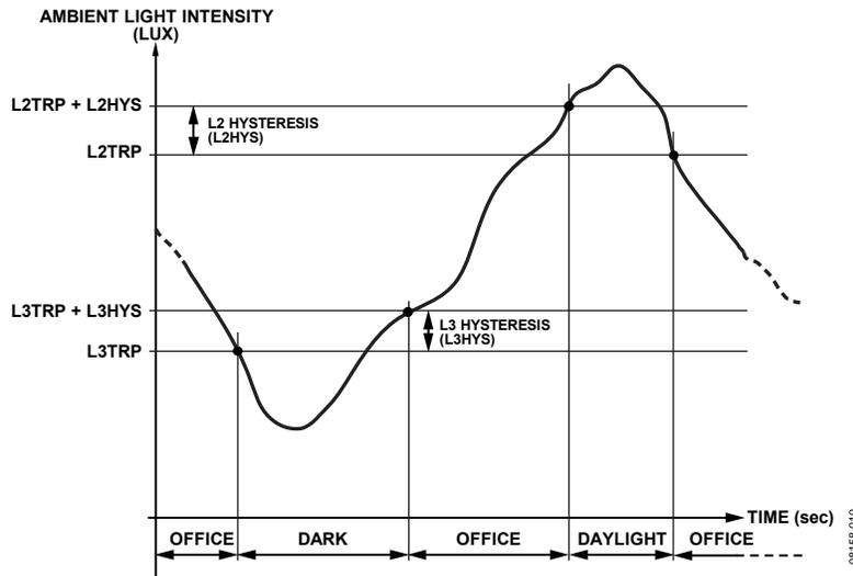
Figure 10. Comparator Thresholds
