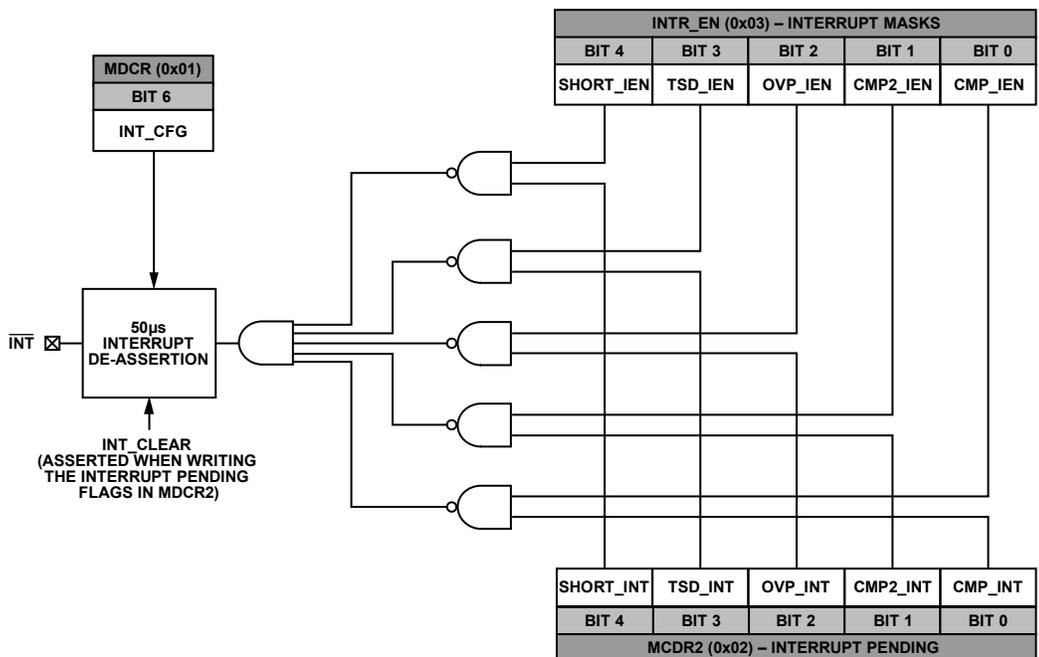
Figure 5. Interrupt Logic
