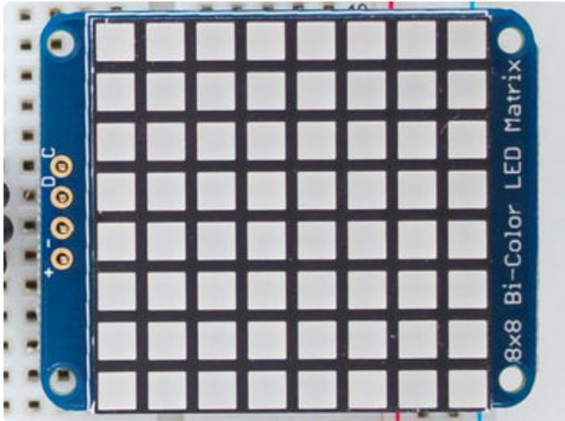
The default orientation for graphics commands on this display places pixel (0,0) at the top-left when the header is at the left and Adafruit logo at the right. To use the matrix as shown above (header at top, logo at bottom), call `matrix.setRotation(3)` before issuing graphics commands.
