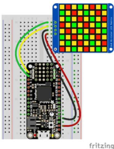
Microcontroller 3V to LED Matrix VIN
