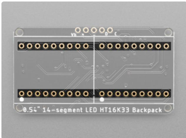
These two rows of through-hole pads are for soldering the alphanumeric LED displays onto the backpack. See the [Assembly page \(https://adafruit.it/11dU\)](https://adafruit.it/11dU) for details on attaching the displays properly.
