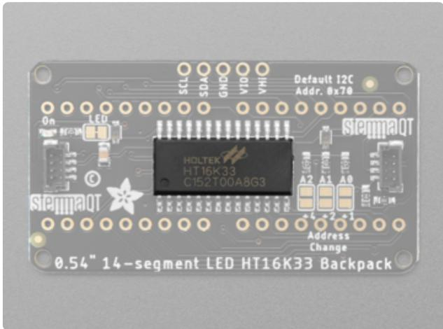
The chip located in the center of the back of the backpack is the HT16K33 matrix driver, which drives the 14-segment LED displays.
