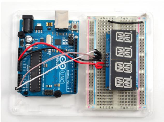
Connect **CLK** to the I2C clock - on Arduino UNO that's Analog #5 (or SCL), on the Leonardo it's Digital #3, on the Mega it's digital #21
