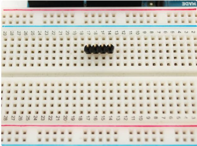
Now you're ready to wire it up to a microcontroller. We'll assume you want to use a 4pin header. You can also of course solder wires directly. Place a 4-pin piece of header with the LONG pins down into the breadboard.
