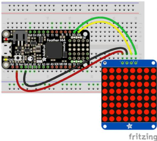
Microcontroller 3V to LED Matrix VIN
