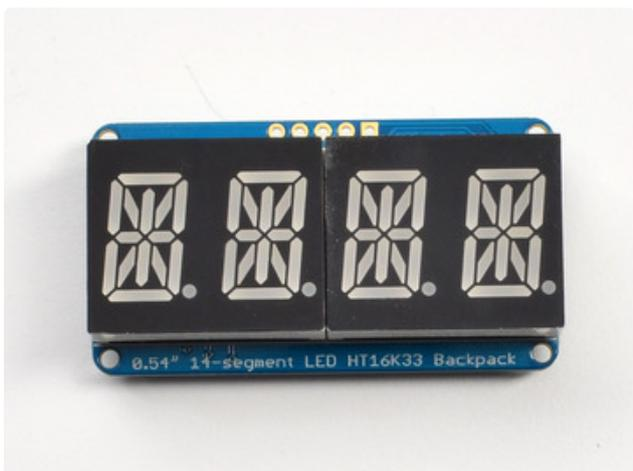
Remove the parts from packaging and place the LED matrices OVER the silkscreen side. **DO NOT PUT THE DISPLAY ON UPSIDE DOWN OR IT WONT WORK!!** Check the image below to make sure the 'decimal point' dots are on the bottom, matching the silkscreen.
