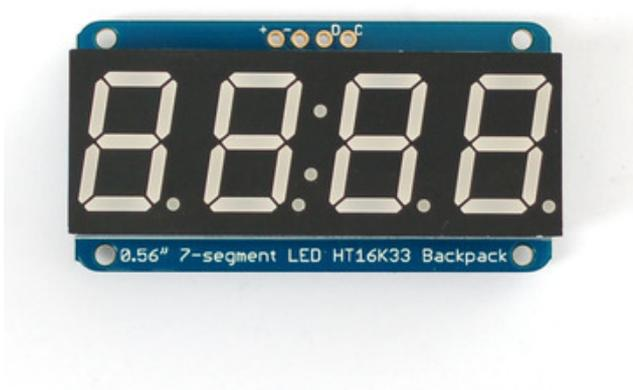
Remove the parts from packaging and place the LED matrix **OVER** the silkscreen side. **DO NOT PUT THE DISPLAY ON UPSIDE DOWN OR IT WONT WORK!!** Check the image below to make sure the 'decimal point' dots are on the bottom, matching the silkscreen.
