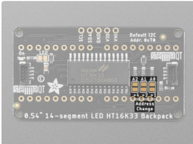
On the back of the board are **three address jumpers**, labeled **A0**, **A1**, and **A2**. These jumpers allow you to chain up to 8 of these boards on the same pair of I2C clock and data pins. To do so, you solder the jumpers "closed" in various combinations by connecting the two pads.
