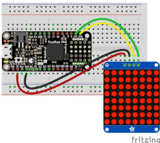
Microcontroller 3V to LED Matrix VIN
