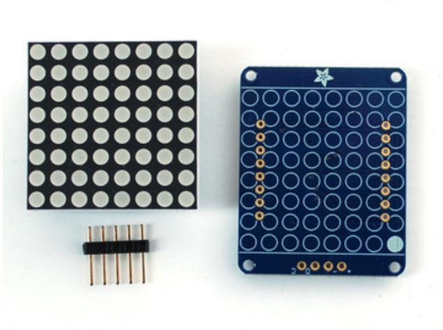
When you buy a pack from Adafruit, it comes with the fully tested and assembled backpack as well as a 8x8 matrix in one of the colors we provide (say, red, yellow or green). You'll need to solder the matrix onto the backpack but its an easy task.
