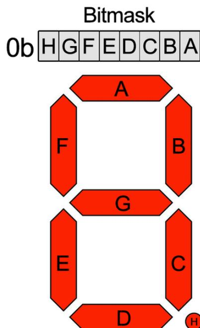
The bitmask is a single 8-bit number that can be passed in as a single Hexidecimal, Decimal, or binary number. This will use a couple different methods to display
