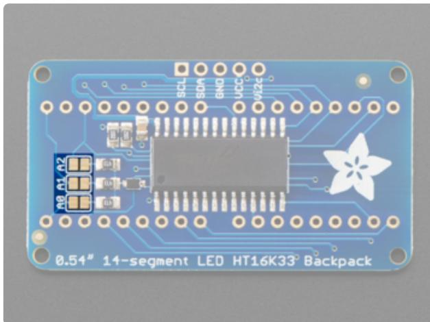
The default I2C address is **0x70**. The other address options can be calculated by "adding" the **A0/A1/A2** to the base of **0x70**.
