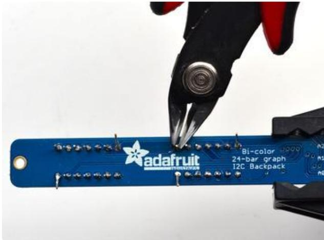
Once soldered, clip each pin. They're quite short and the pins are thicker than usual, so do this over/inside a trash bin so that the pins don't fly off and hit you or your pets.
