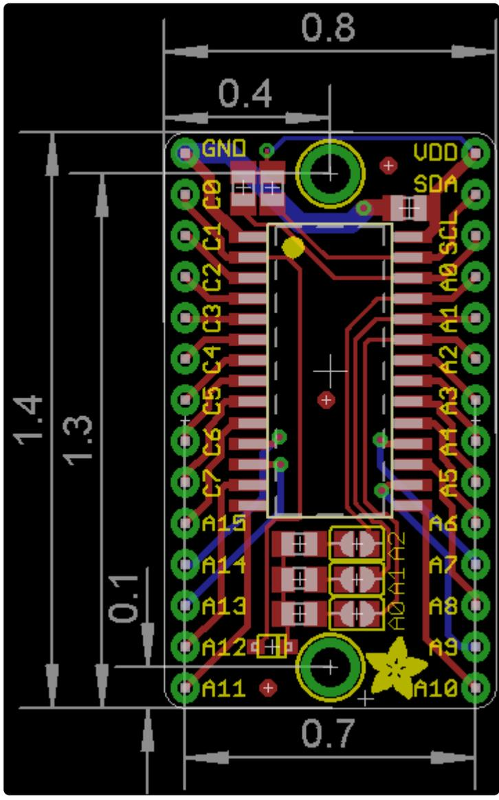
NOTE - The silkscreen labels for the A0/A2 header pins are swapped. The silkscreen labels for the solder pads are correct.
