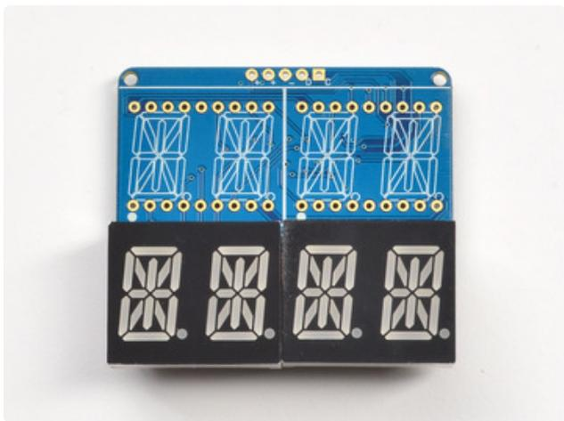
When you buy a pack from Adafruit, it comes with the fully tested and assembled backpack as well as two dual 14-segment display in one of the colors we provide (say, red, yellow, blue or green). You'll need to solder the matrix onto the backpack but it's an easy task.
