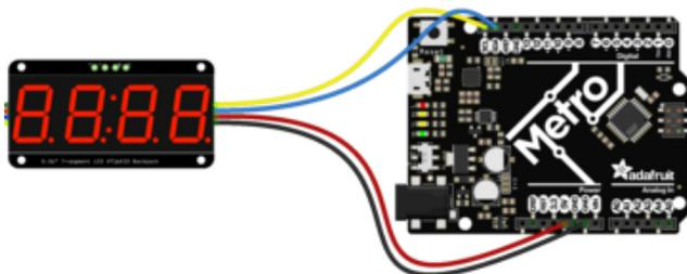
Backpack + (VCC) to microcontroller 5V (if using a board with 5V logic, otherwise use 3V for boards with 3V logic) (red wire)
