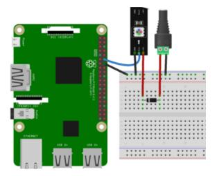
Pi pin 18 to NeoPixel DIN. 1N4001 diode cathode (side with the stripe) to NeoPixel 5V.
