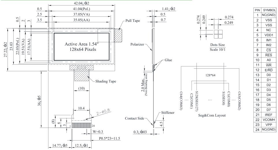
The non-specified tolerance of dimension is ;  $\dot{\Omega}3 \text{ mm}$ .
