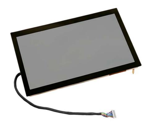
LCD Application Kit, including 10" WXGA (1280x800) LCD panel with PCAP touch
